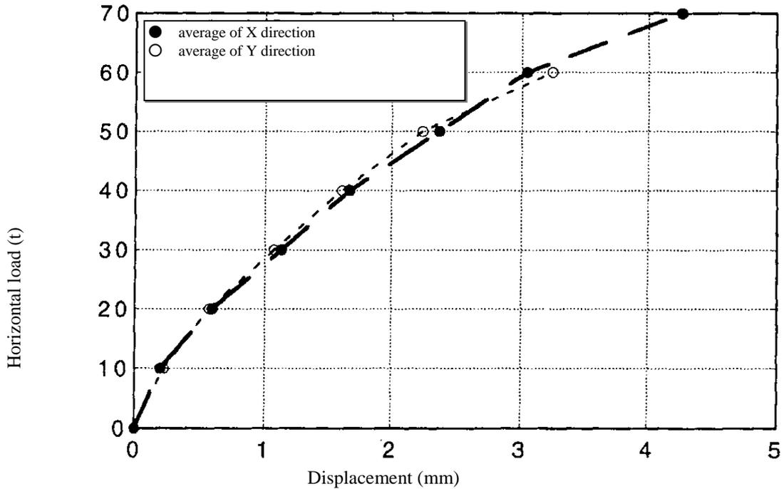
Figure 5.6.1: Load-displacement curve of the seismic isolation bearing
