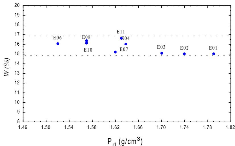
**Fig 1: The  $w$  and  $\rho_d$  of specimens used in dynamic modulus test of compacted loess**
