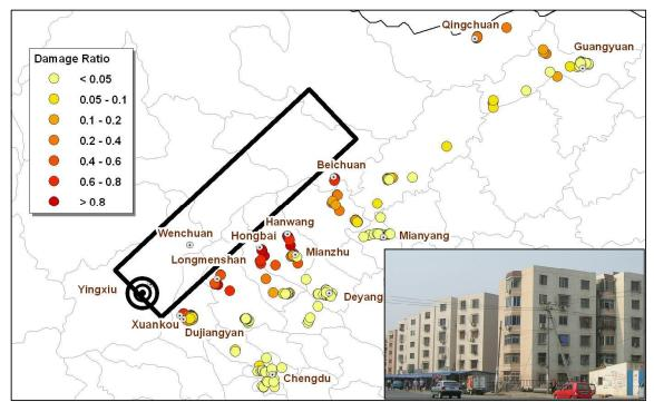
Figure 2: Spatial distribution and damage severity of assessments of Mid-rise CM buildings
