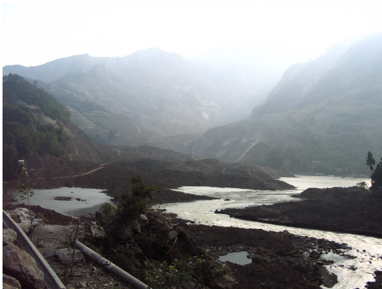
Photo 3 Landslide on alpine gorge region ( 105^{\circ}17'51.1'' , 32^{\circ}32'22.9'' ) , the bond between soil layer and rock body is lost, which caused by asynchrony vibration
