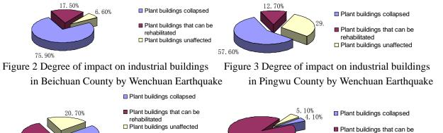
Figure 4 Degree of impact on industrial buildings in Anxian County by Wenchuan Earthquake
