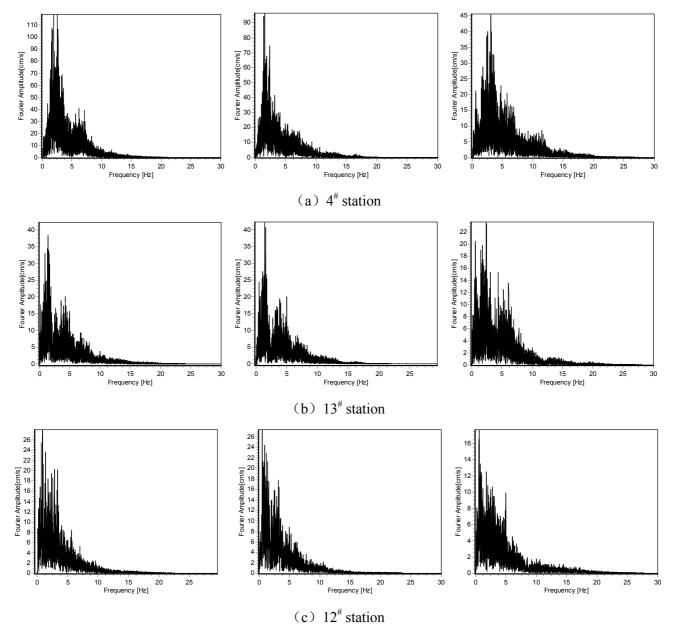
Figure 8 Fourier spectrum in transverse, longitudinal and vertical direction during the 5.12 Wenchuan Earthquake
