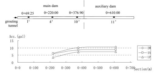
Figure 7 Distribution of acceleration on crest along dam axis during the earthquake on May 23, 2007
