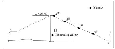
Figure 3 The disposal of strong motion instruments on the biggest section of the YeLe dam
