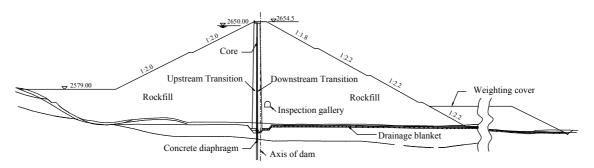
Figure 1 Maximum transverse cross section of the Yele Dam
