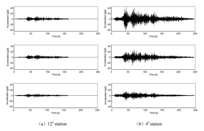
Figure 4 Time history of transverse, longitudinal and vertical accelerations during 5.12 Wenchuan Earthquake
