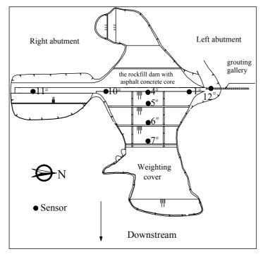
Figure 2 The planar disposal of strong motion instruments of the YeLe dam
