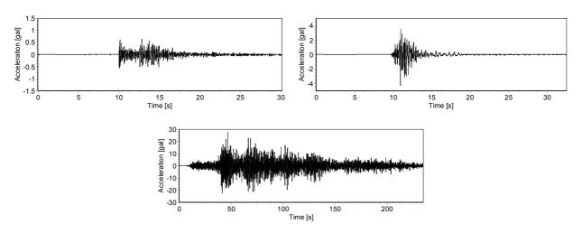
Figure 5 Time history of transverse acceleration at  $5^{\#}$  station during the three earthquakes
