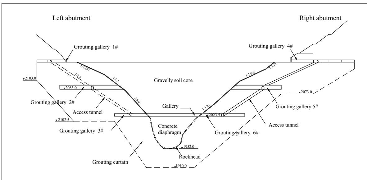
Figure 2 Maximum longitudinal cross section of the Yele Dam
