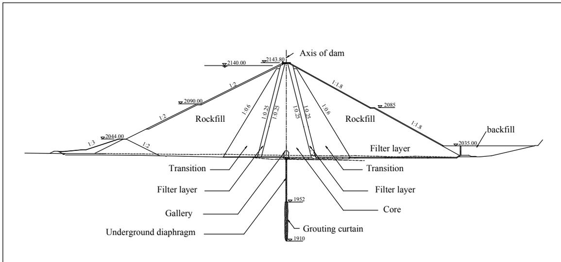
Figure 1 Maximum transverse cross section of the Yele Dam
