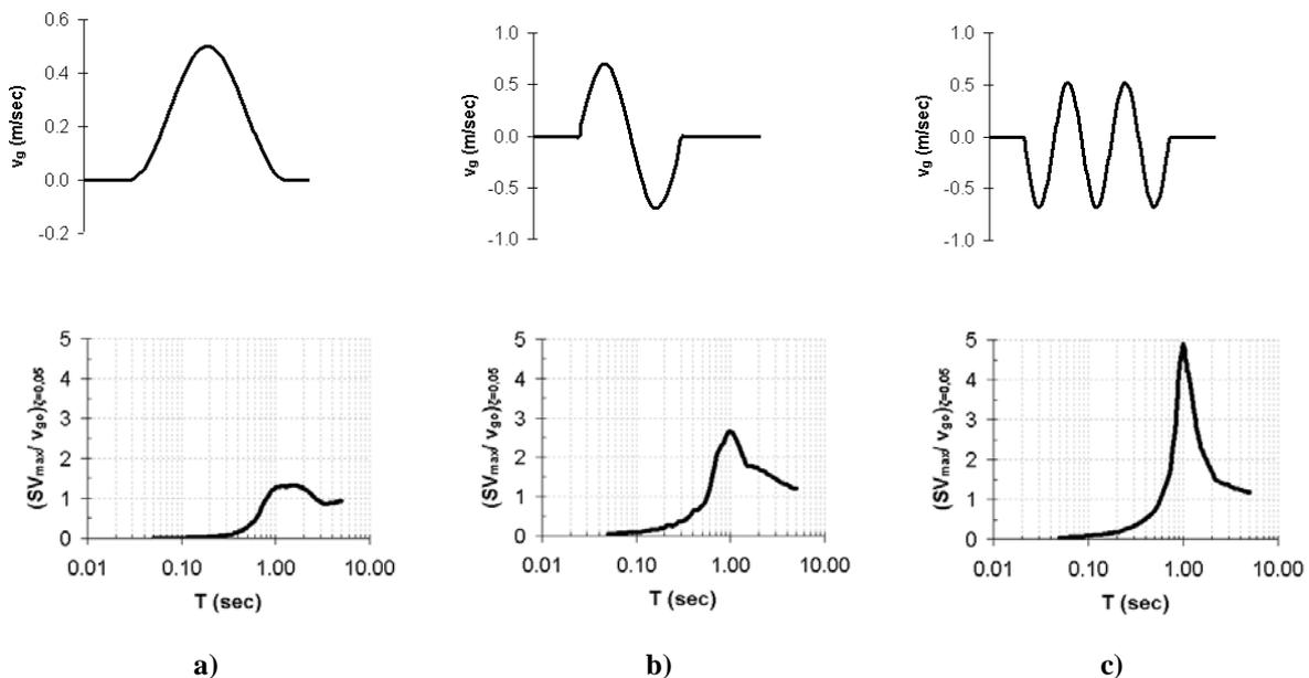
Figure 3 Schematic representation of velocity time history and spectral amplification for: a) Pulse Type-A; b) Pulse Type-B; and c) Pulse Type-C<sub>2</sub>
