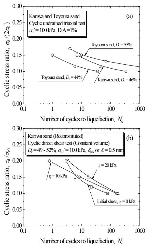
Figure 9 Effects of initial shear on liquefaction resistance in Kariwa sand: (a) Cyclic undrained triaxial test, (b) Cyclic direct shear test under constant volume
