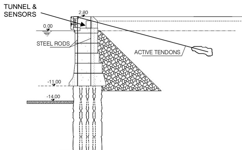
Figure 1 San Giorgio Pier – East wall cross section and location of sensors
