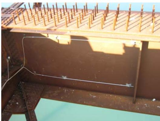
Figure 5 Positioning of the SOFO sensors on the girder web
