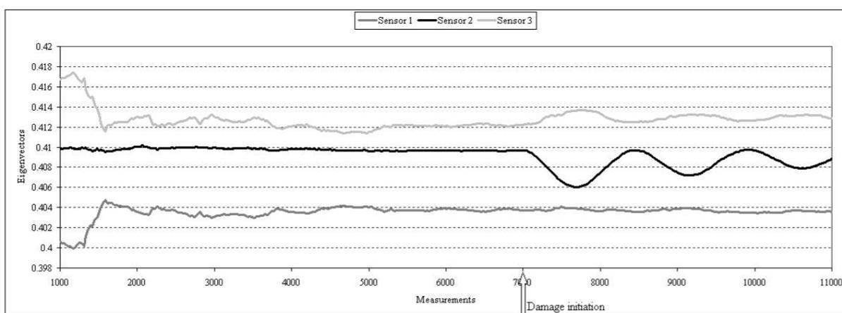
Figure 7 POD eigenvectors for 1 element stiffness reduction of 50% inside sensor 2 base length
