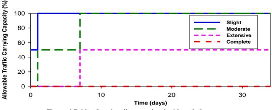
Figure 4 Bridge functionality associated with each damage state
