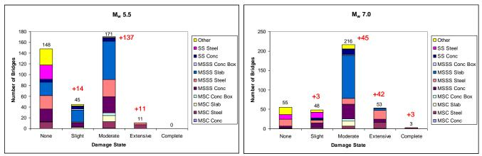
Figure 5 Damage state distribution by bridge type and damage state for  $M_w$  5.5 and 7.0 events.
