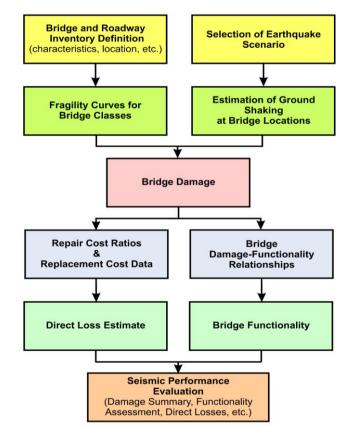
Figure 1 Schematic of general seismic risk assessment methodology applied
