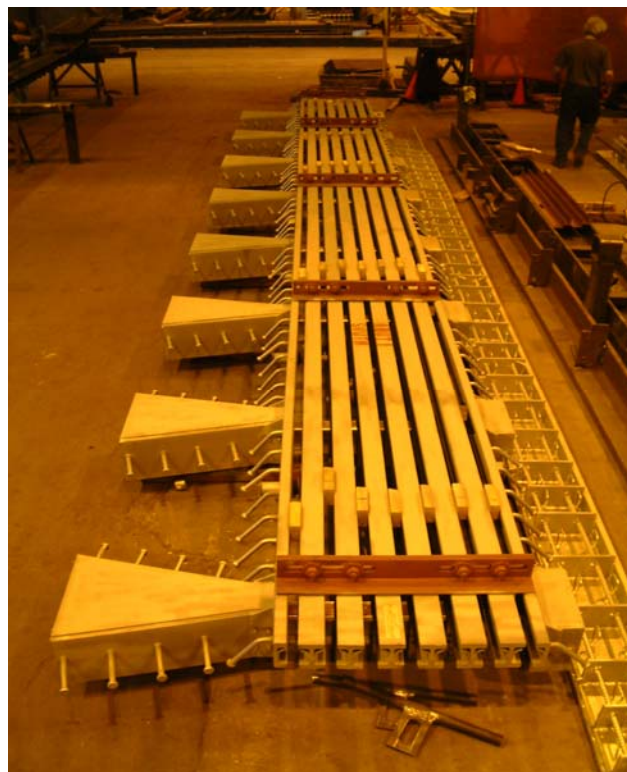
Fig. 8 (swiveling capable boxes to permit both longitudinal and transverse movements)
