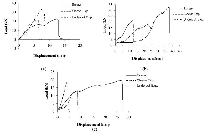
Figure 4 Static test results (a) Typical anchor tensile force-axial displacement, (b) Anchor shear force-lateral displacement, and (c) Anchor resultant force-resultant displacement under combined load
