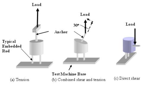
Figure 2 Typical test set-up and applied loadings
