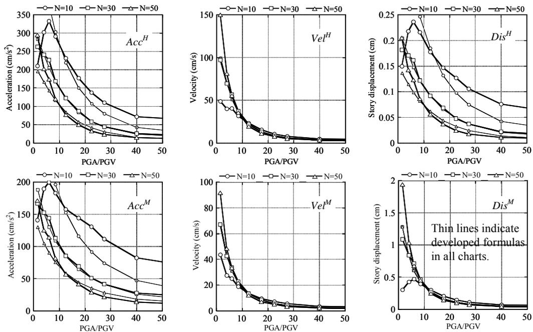
Figure 4 The relationships between  $PGA/PGV$  and  $R^{H,M}$  for a RC building with  $N=10, 30, 50$
