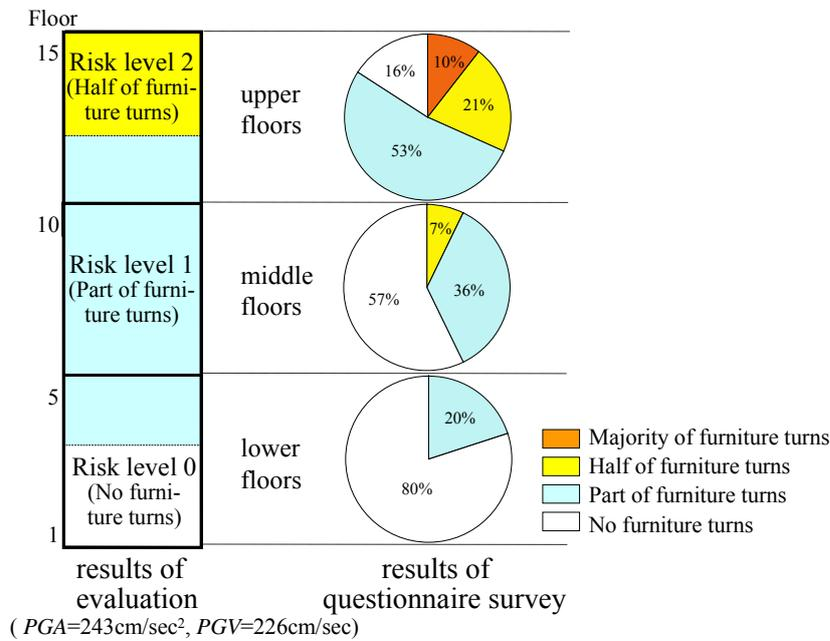
Figure 7 Estimated overturning ratios of furniture in a 15-story RC building in comparison with the actual overturning ratios surveyed by questionnaires after the 2005 West off Fukuoka earthquake (March 20, 2005)
