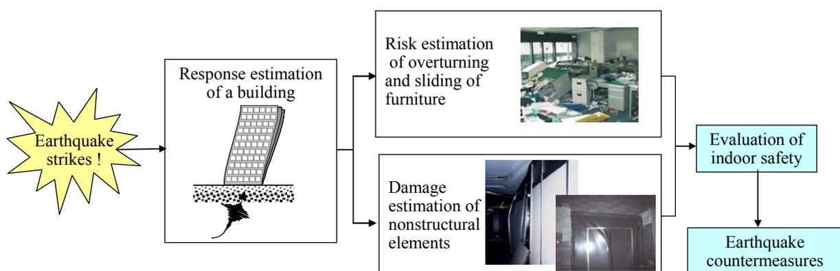
Figure 1 The flow of the indoor safety evaluation
