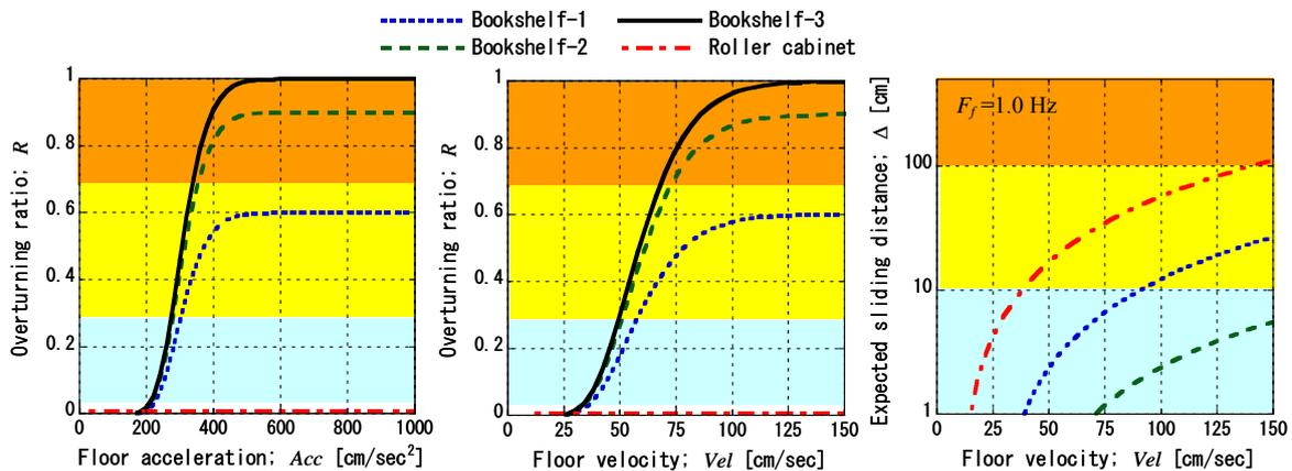
Figure 5 The relationships between floor responses and overturning ratios or sliding distance of furniture
