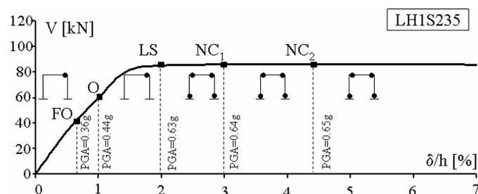
Figure 3 Example of pushover curve for the determination of the earthquake-induced damage
