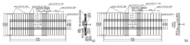
Figure 2 Slab reinforcement of a) a prefabricated lattice girder slab, b) a profiled steel sheeting slab
