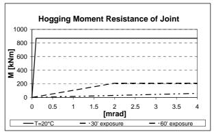
Figure 10. Moment-rotation relationship of a joint as a function of time at different fire exposures
