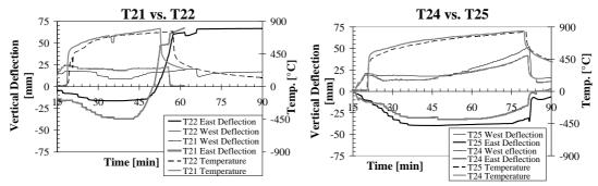
Figure 7 Fire test results: a) comparison between pre-damaged (T21) and undamaged (T22) steel sheeting specimens; b) comparison between pre-damaged (T24) and undamaged (T25) precast specimens
