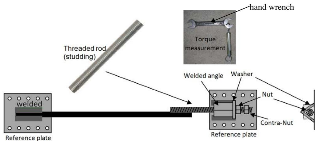
Figure 1 Schematic representation of post tensioning mechanism using bolts.
