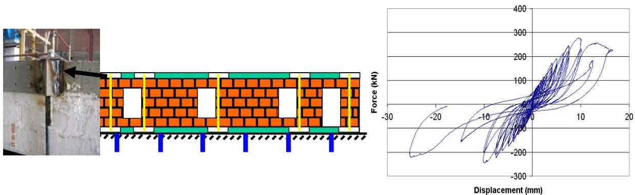
Figure 6 Load versus deflection curve of the vertically post-tensioned masonry house
