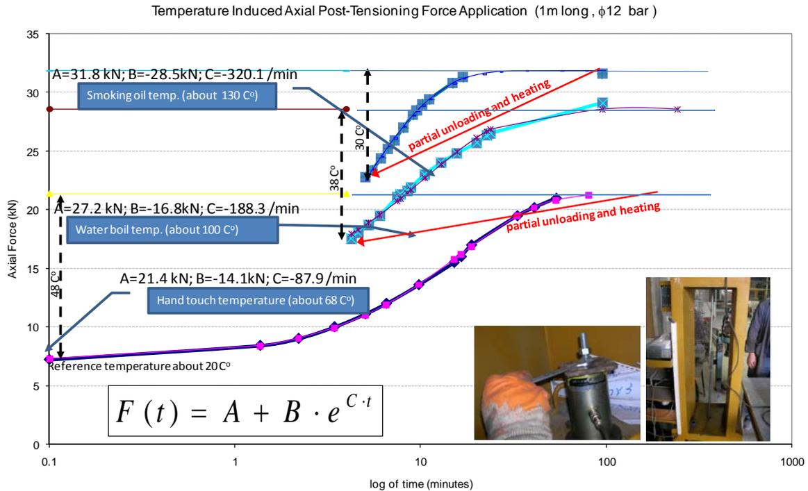
Figure 2 Temperature induced post-tensioning force application tests
