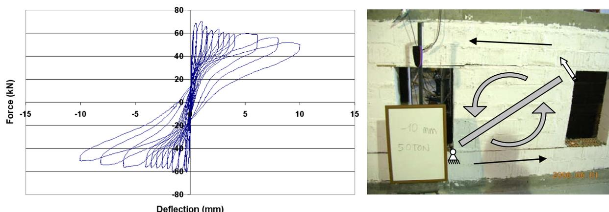
Figure 4 Load versus deflection curves of original (nominal) house
