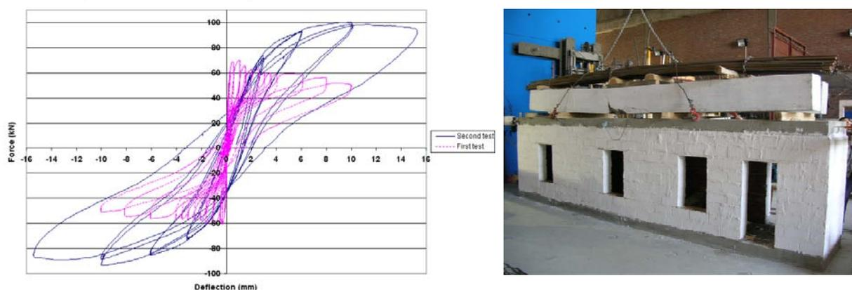
Figure 5 Load versus deflection curves of the original house with 5000kg mass on the roof
