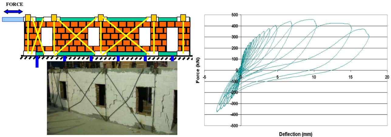
Figure 7 Load versus deflection curve of the vertically and diagonally post-tensioned masonry house
