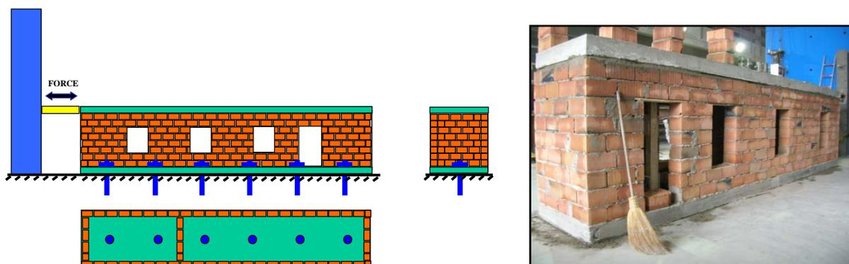
Figure 3 Half-scale brick masonry house model constructed in the laboratory
