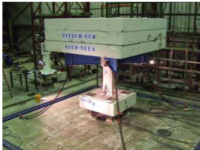
Photo 1 Setup of Column Model on the Shake Table
