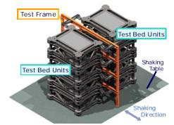
Figure 6 Multipurpose TestBed in E-Defense
