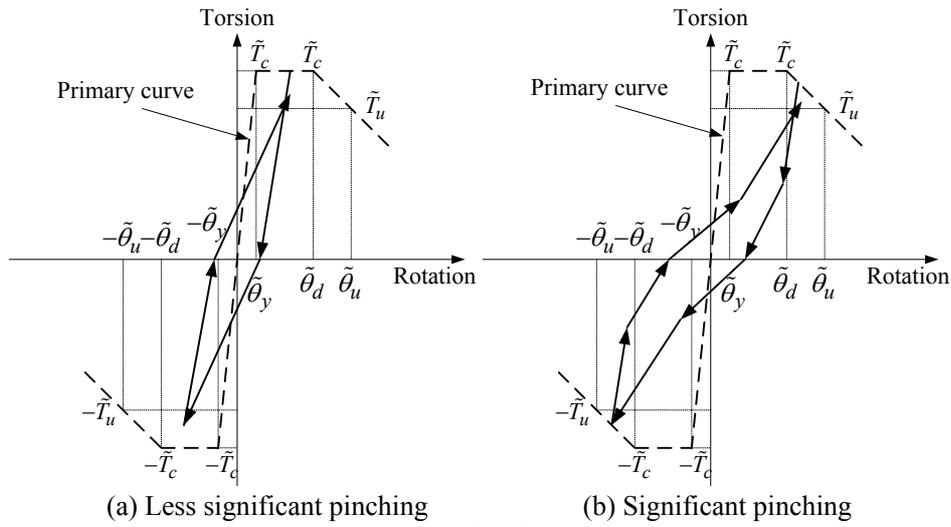
Fig. 5 Nonlinear torsional hysteretic model
