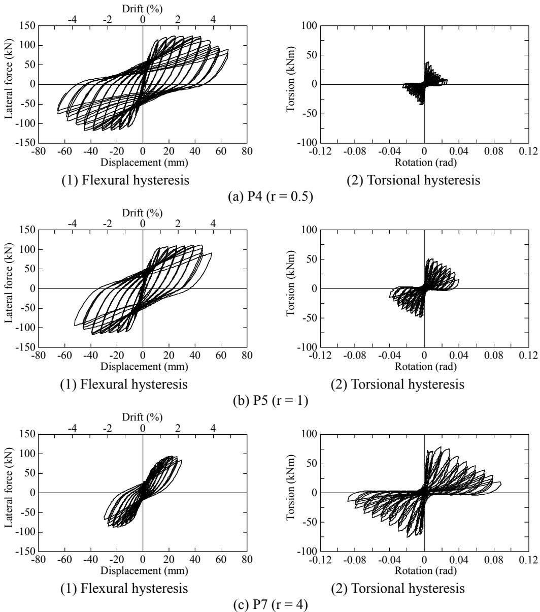
Fig. 3 Flexural and torsional hysteretic curves of columns under combined bending and torsion.
