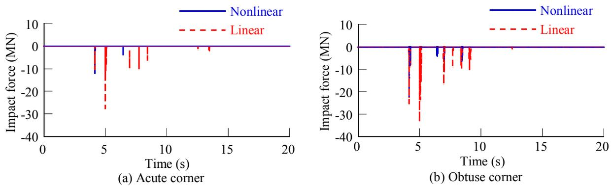
Fig. 8 Impact force between deck and abutment A2 ( x direction )
