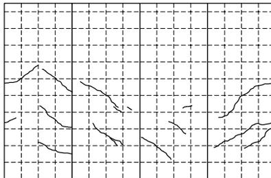
Fig. 11 Crack modes of a column loaded under  $r = 1.0$  ( $\theta = 0.005$  rad and  $\Delta = 0.5\%$ )
