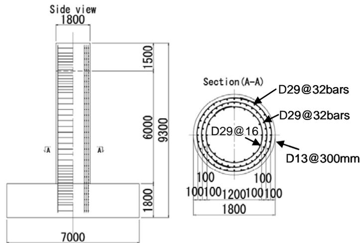
Figure 1 Column built 1960-1970s which fails in Flexure (C1-1 column)
