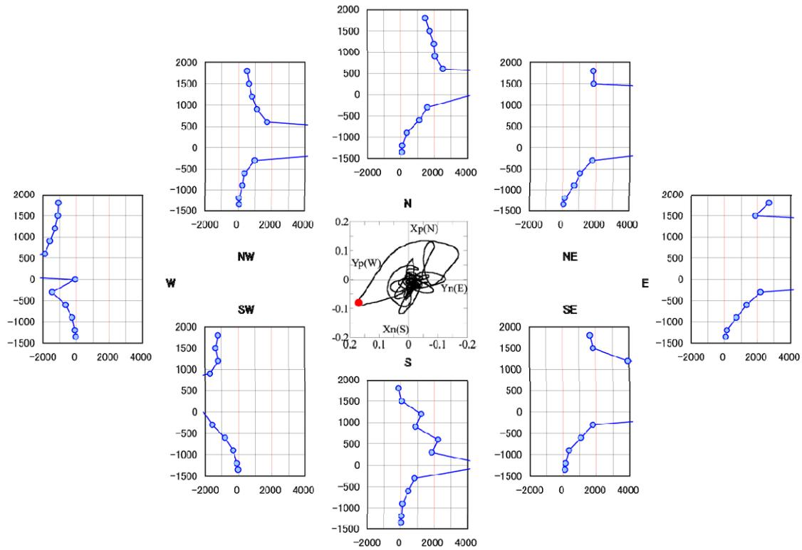
Figure 5 Strains of Outer Longitudinal Bars at 6.9 sec during the First 100% E-Takatori Ground Acceleration Excitation
