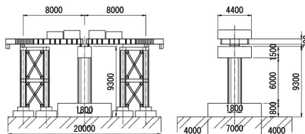
Figure 2 Setup of Model
