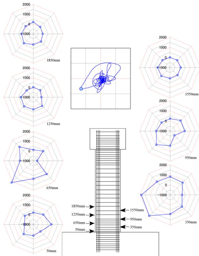
Figure 6 Strains of Ties at 6.9 sec during the First 100% E-Takatori Ground Acceleration Excitation
