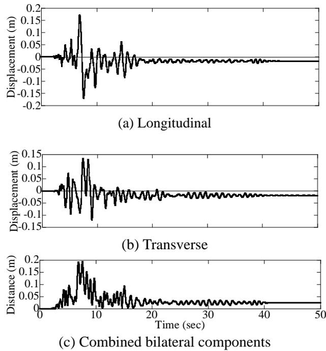
Figure 4 Response Displacement of C1-1 at the Top during the First 100% E-Takatori Ground Acceleration Excitation
