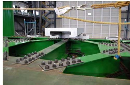
Photo 5 Movable Bearing and 2 Side Sliders
