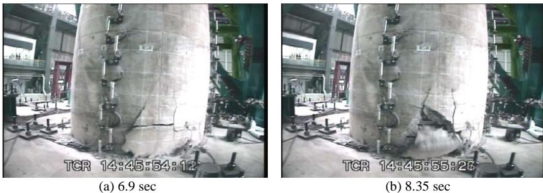
Photo 6 Progress of Failure of C1-1 during the First 100% E-Takatori Ground Acceleration Excitation
