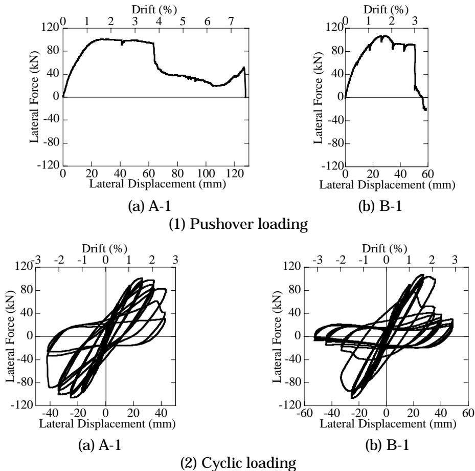
Figure 4 Lateral Force vs. Lateral Displacement under Pushover and Cyclic Loadings
