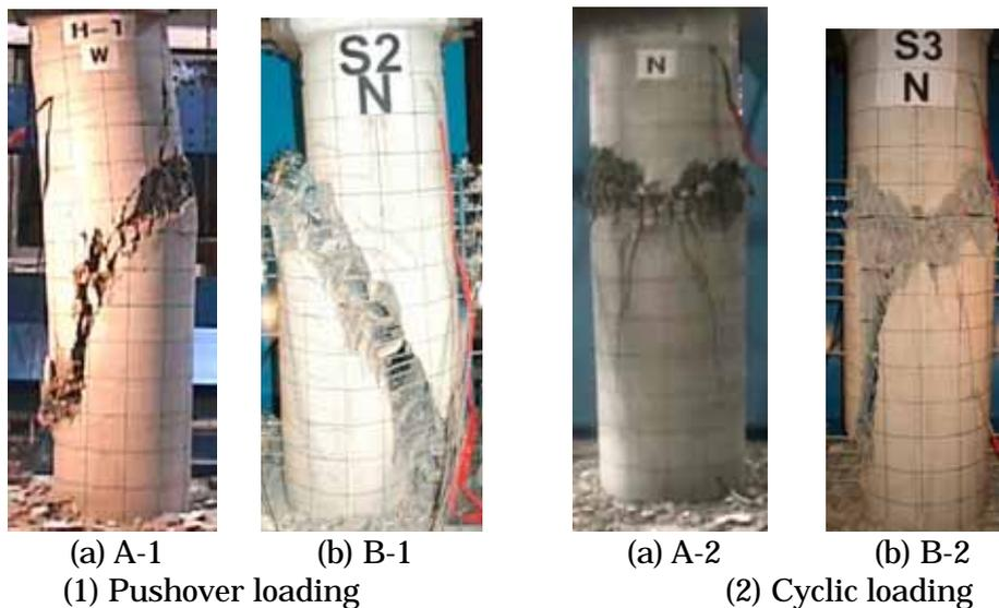
Figure 3 Damage after Pushover and Cyclic Loadings
