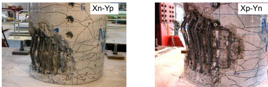
Figure 7 Failure mode of flexural failure specimen
