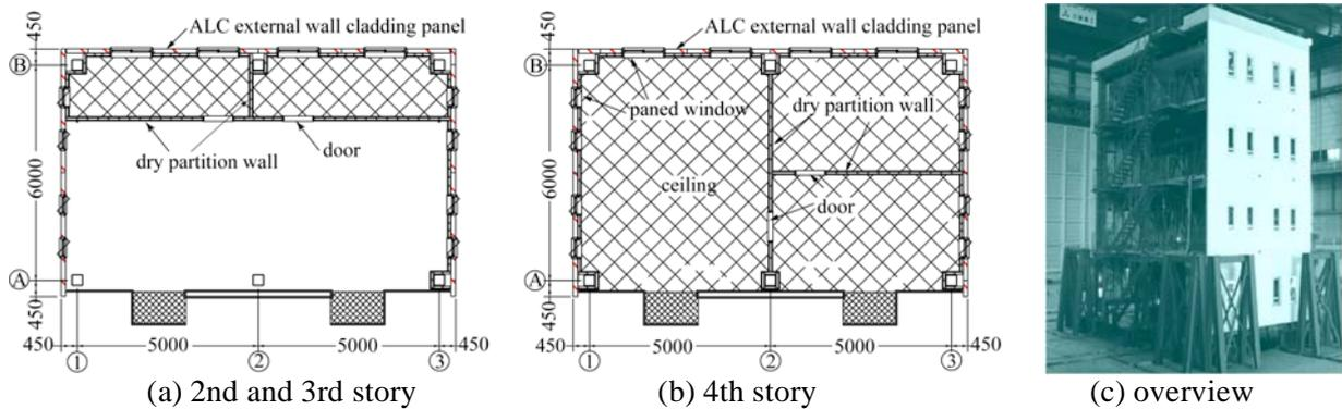
Figure 2 Plan and non-structural components (unit: mm)
