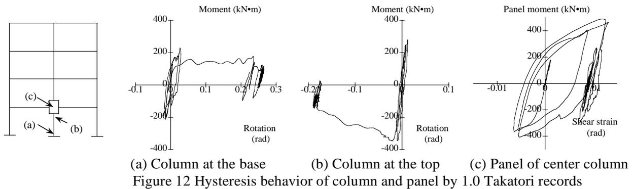
(a) Column at the base (b) Column at the top (c) Panel of center column
