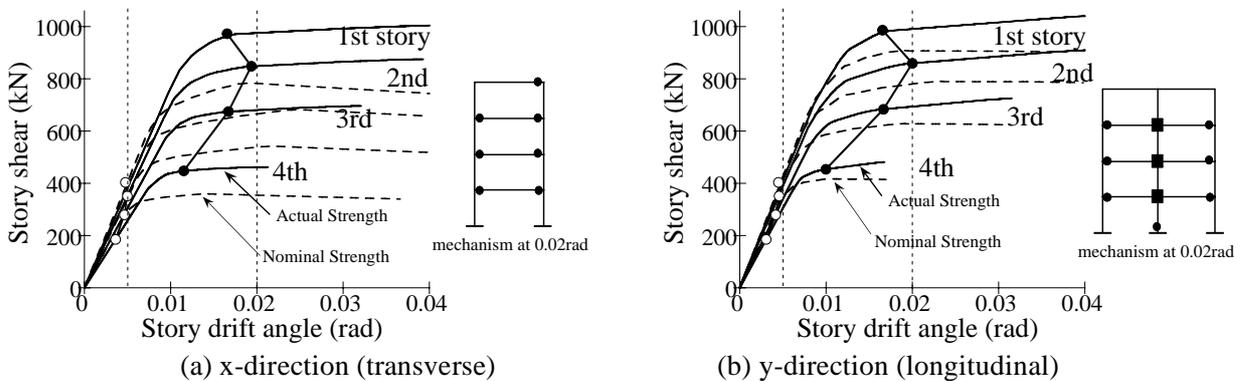
Figure 3 Story shear versus story drift relationships obtained from pushover analyses
