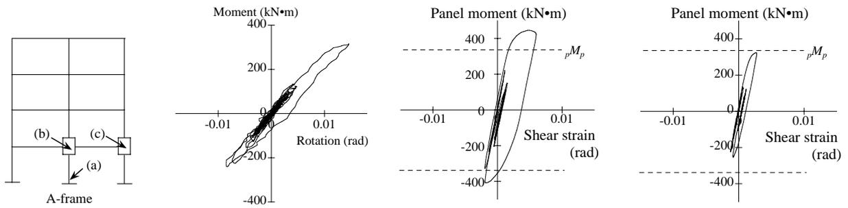
(a) Column at the base (b) Panel of center column (c) Panel of side column
