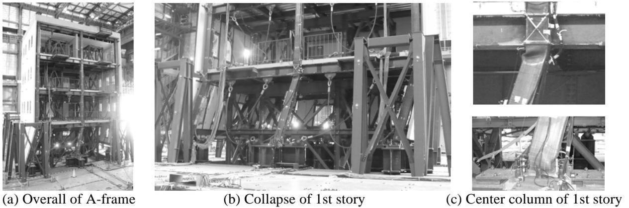
Figure 9 Collapse of specimen after test by 1.0 Takatori records
