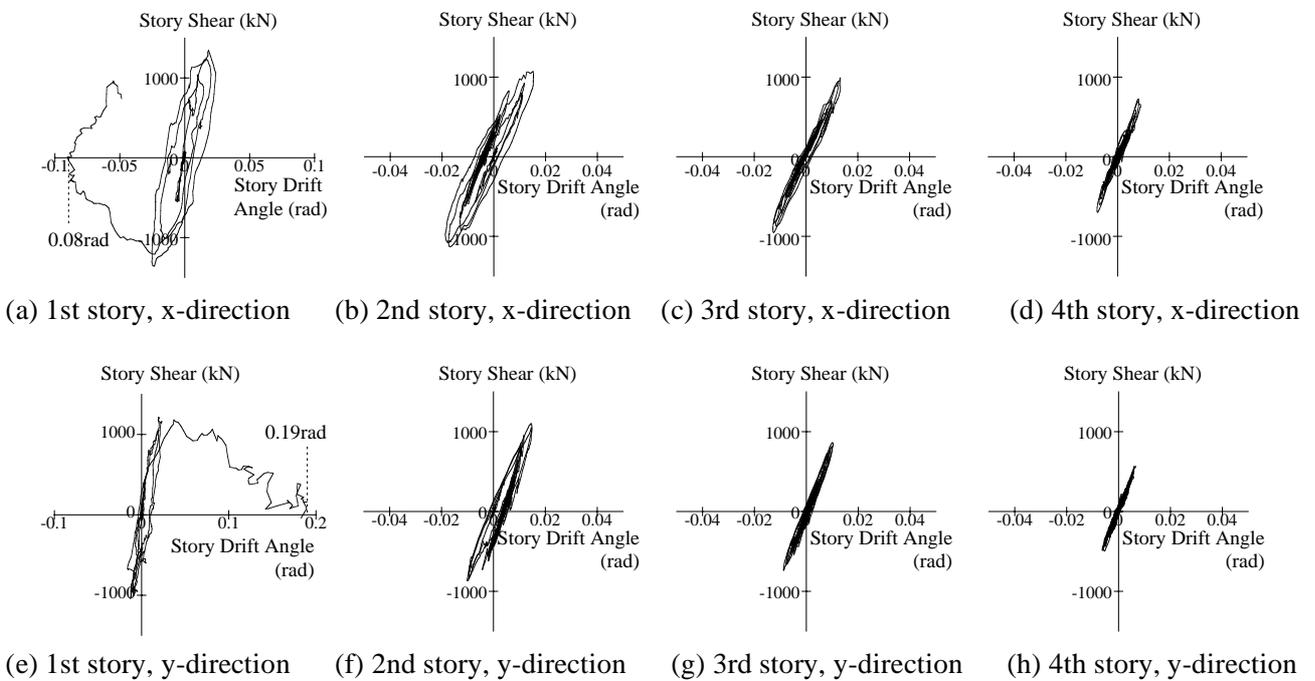
Figure 10 Story shear force and inter-story drift relationships by 1.0 Takatori records
