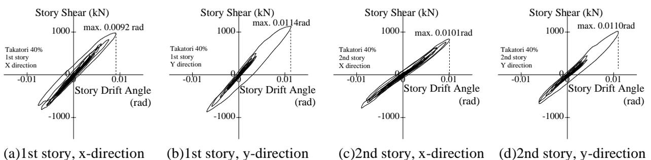
Figure 4 Story shear force and inter-story drift relationships by 0.4 Takatori records
