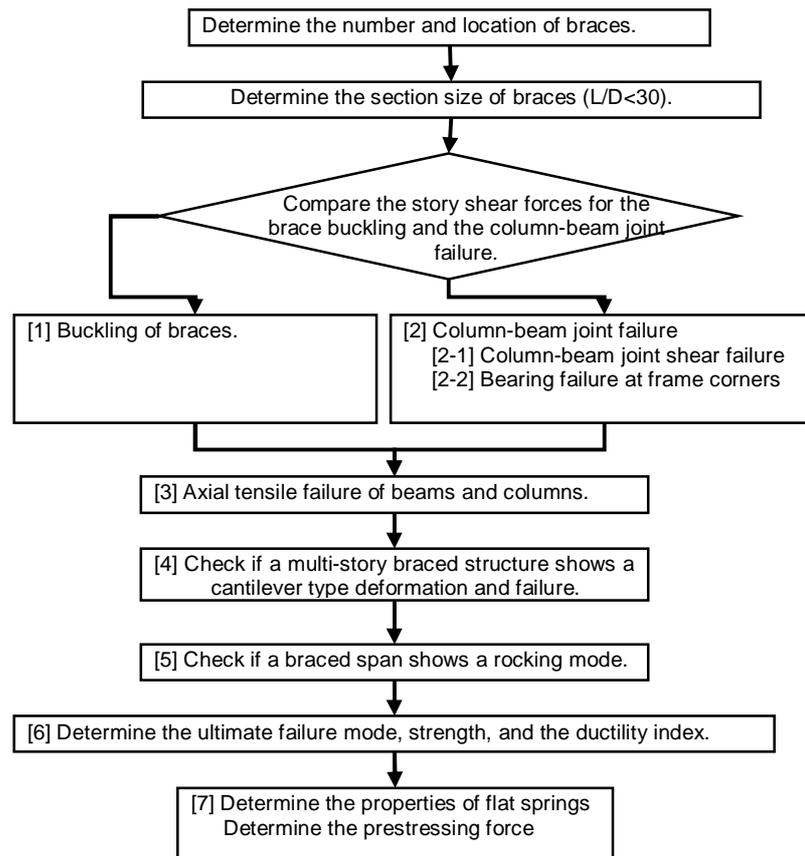
Fig. 10. Design flow of prestressed CFT and FRC braces
