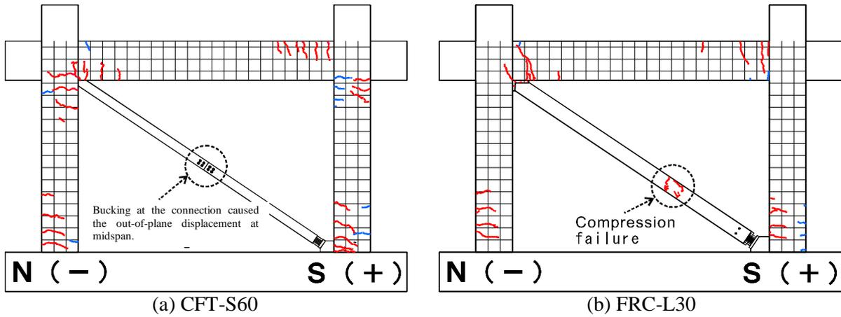
Fig. 5. Observed damage at R=0.8%
