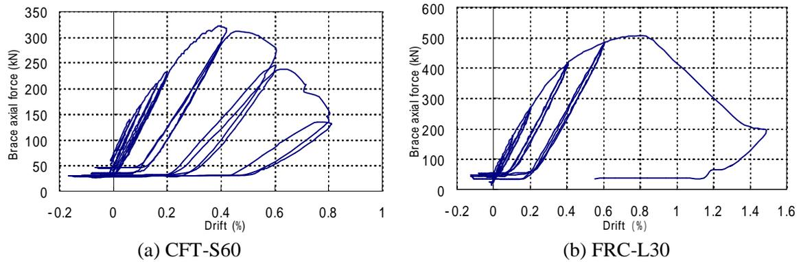
Fig. 7. Axial compressive force of the brace – drift relations
