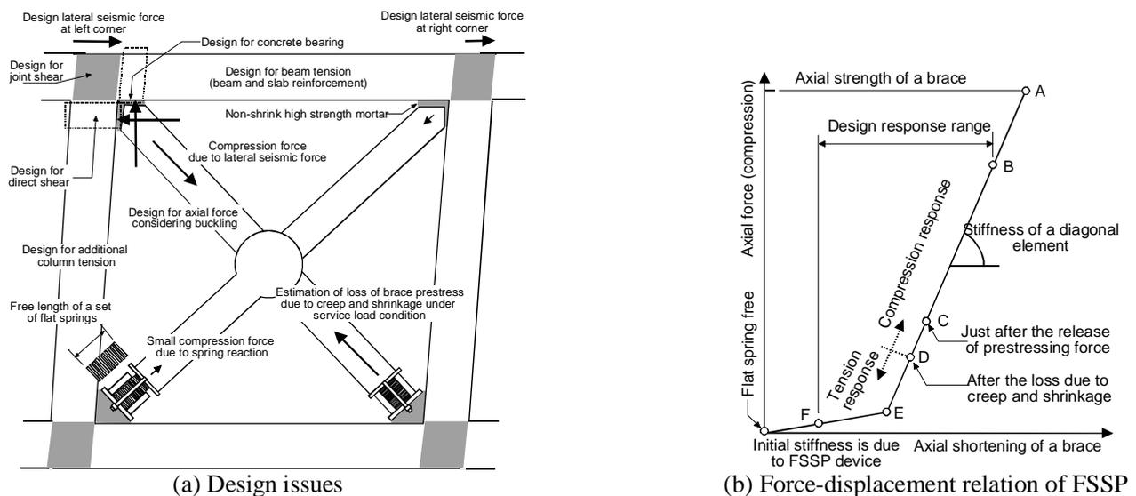
Fig. 9. Major design issues for a proposed bracing system
