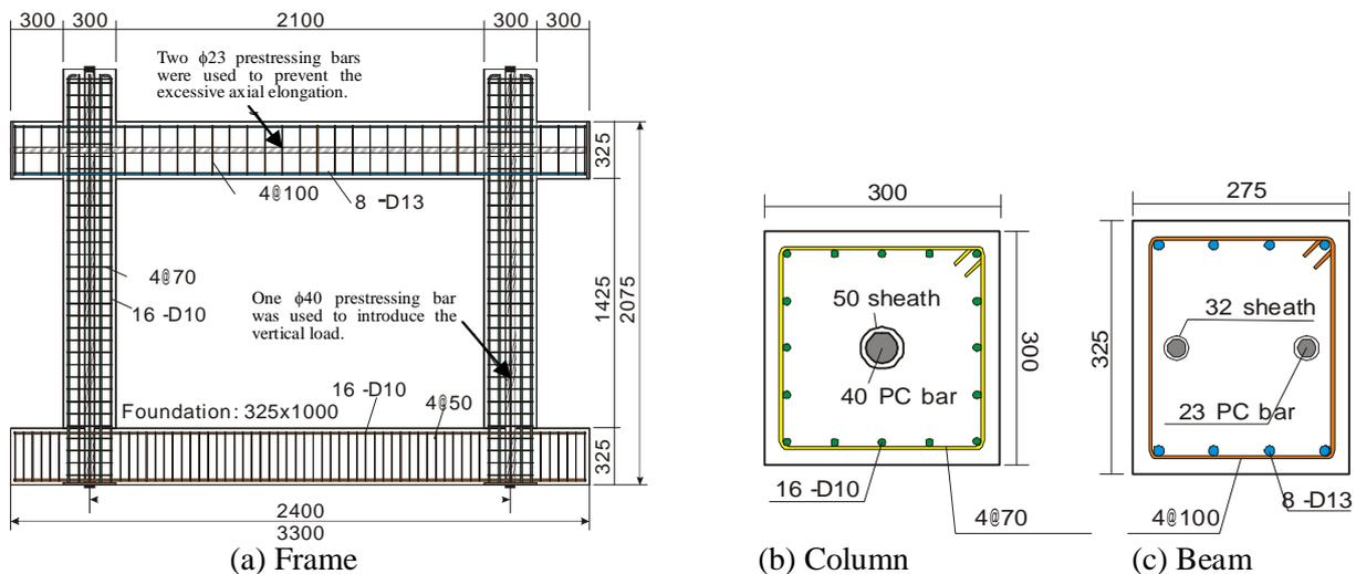
Fig. 3. Reinforcing bar arrangement of the portal frame
