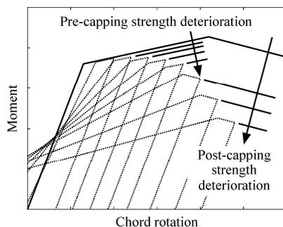
Figure 11 Strength deterioration in the Ibarra's model
