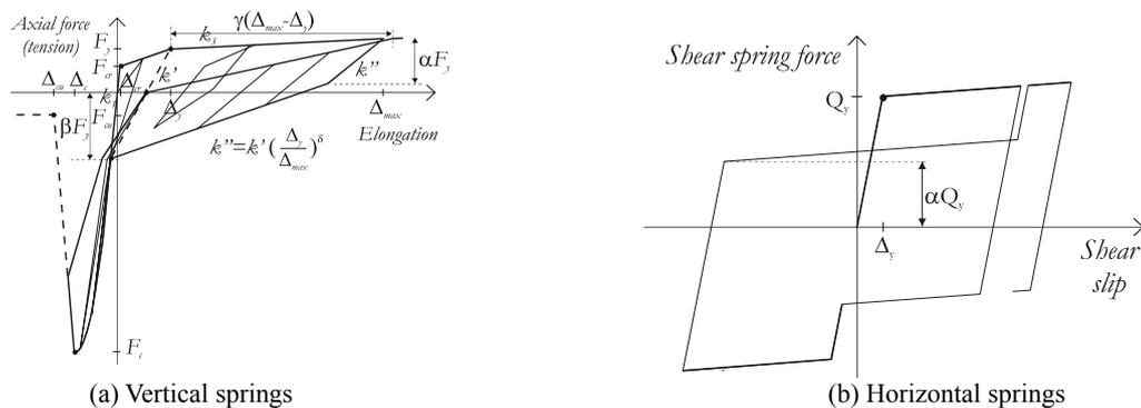
Figure 2 Hysteretic rules controlling the springs in the MVLEM
