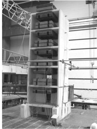
Figure 5 Coupled structural wall, designed according to the Slovenian building practice
