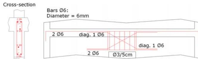
Figure 7 Reinforcement in the coupling beams
