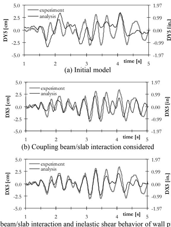
Figure 9 Top displacement response history in the direction of the flange wall with openings
