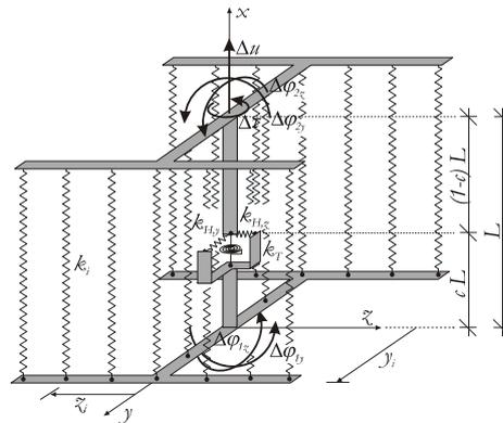
Figure 1 3D multiple-vertical-line-element model (MVLEM-3D)
