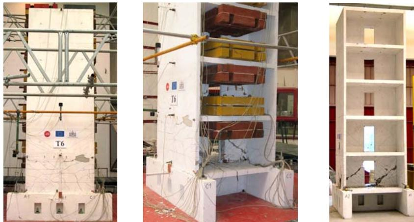
Figure 8 Damage in the coupled wall after the last test
