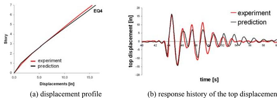
Figure 4 Comparison of the predicted response and experimental results for the NEES building
