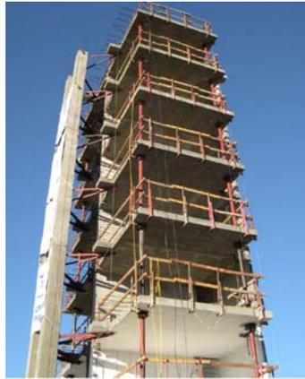
Figure 3 The set-up of the NEES 7-story building slice at UC San Diego
