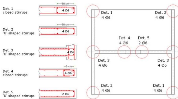
Figure 6 Reinforcement details for the piers of the coupled structural wall
