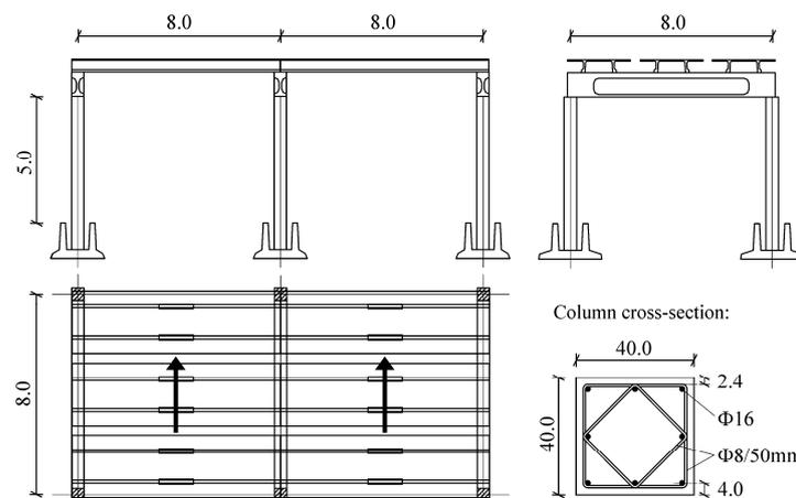
Figure 10 Precast industrial building tested at ELSA, Ispra, Italy
