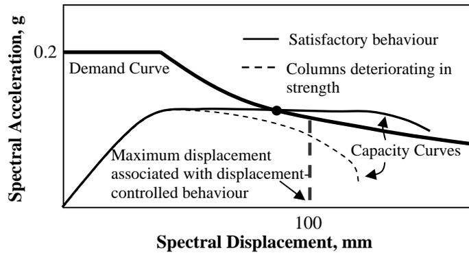
Figure 2 Schematic view of acceleration-displacement response spectrum diagram
