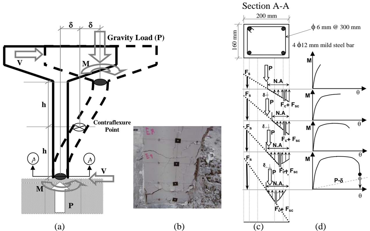
Figure 6 Flexural failure mechanism of a column ; (a) a column supporting a soft-storey building subject to lateral force, (b) photo of a column failed in flexure (c) stress diagram at the critical section of a column subject to increasing lateral deformation, (d) moment – rotation ( $M-\theta$ ) relationship at the critical section of a column.
