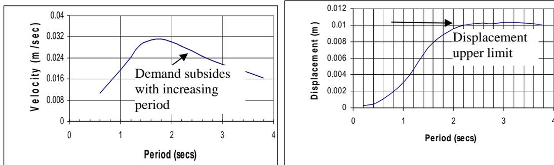
(b) Velocity response spectrum (c) Displacement response spectrum
