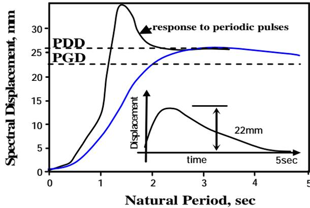
Figure 4 Displacement response spectrum for single and periodic pulses
