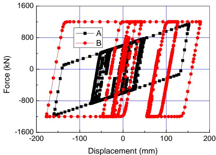
Figure 4.1 Hysteresis loops from seismic analysis
