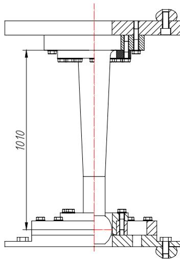
Figure 2.1 Sketch of equipping a damper
