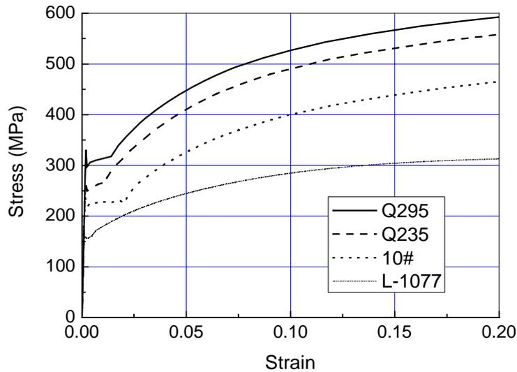
Figure 2.2 Constitutive curves from tensile tests
