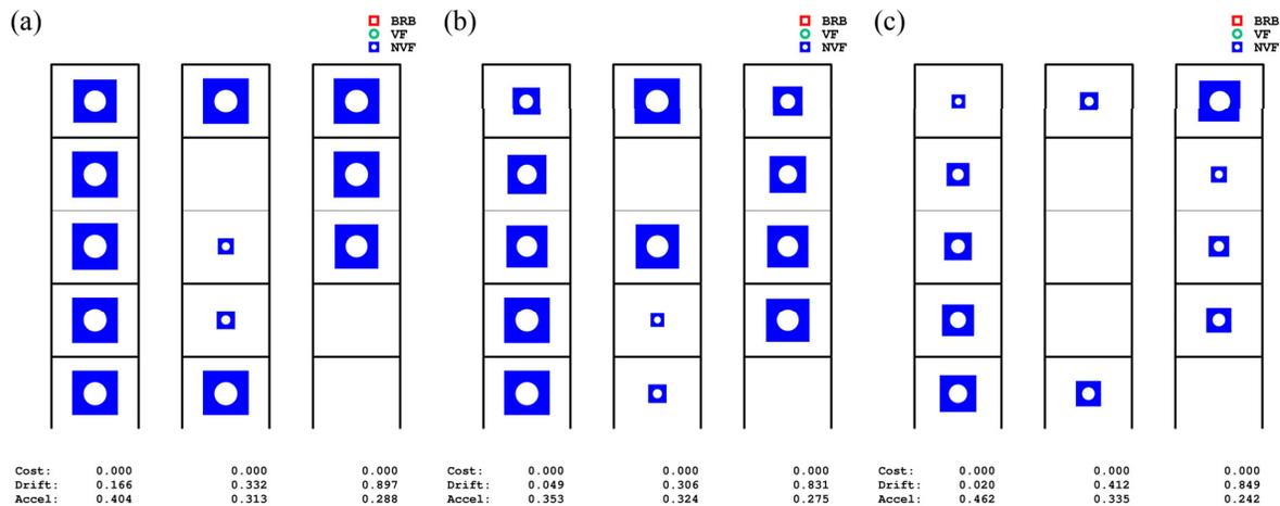
Figure 4 Five story yielding shear frame Pareto front damper distributions for  $\kappa = 10$ : (a) NVF with  $\nu = 1.0$ ; (b) NVF with  $\nu = 0.6$ ; (c) NVF with  $\nu = 0.2$
