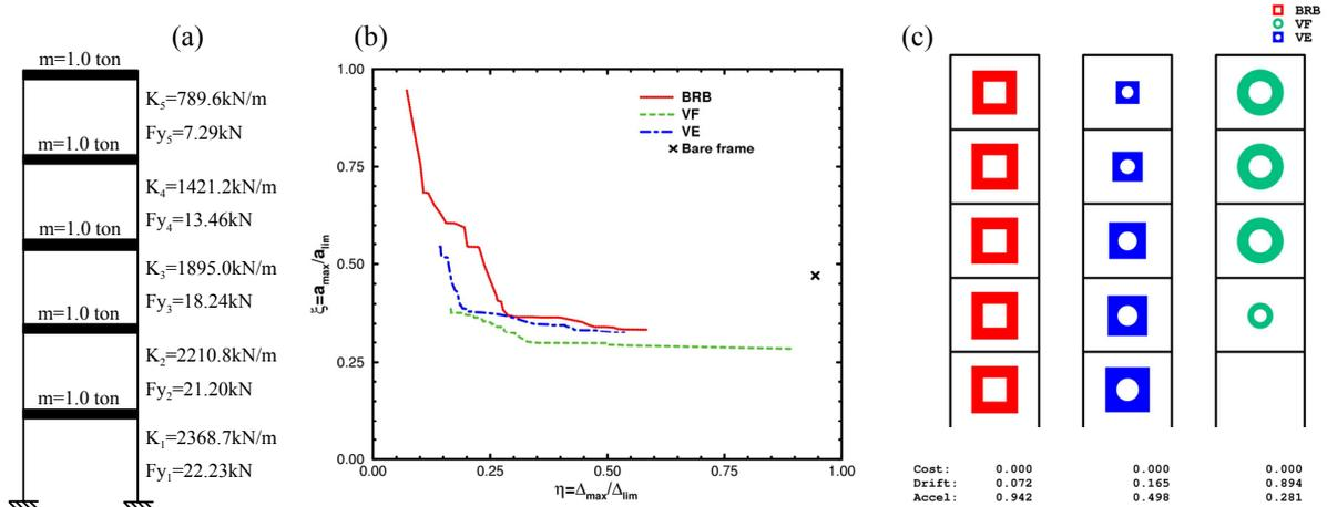
Figure 2 Five story yielding shear frame: (a) Model definition; (b) Pareto front for BRB, VF and VE dampers; (c) Optimal damper distributions
