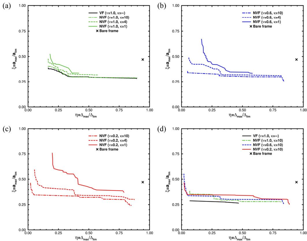
Figure 3 Five story yielding shear frame: (a) Pareto front for NVF with  $\nu = 1.0$  and variable  $\kappa$ ; (b) Pareto front for NVF with  $\nu = 0.6$  and variable  $\kappa$ ; (c) Pareto front for NVF with  $\nu = 0.2$  and variable  $\kappa$ ; (d) Pareto front for NVF with extended damper range and  $\kappa = 10$
