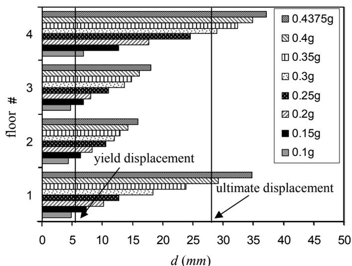
Figure 4 Distribution of BRB maximum displacements for different values of BRB ductility
