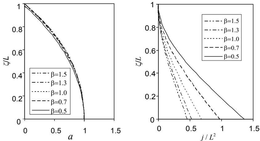
Figure 1 Trends of shear and flexural stiffness distributions along the cantilever.
