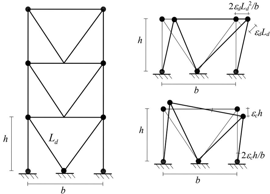
Figure 2 V-bracing system: geometry (a); floor shear deformation and floor curvature (b).
