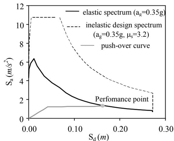
Figure 3 Static push-over analysis results
