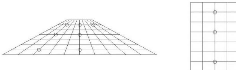
Fig 2 Arrangement scheme of acceleration sensors
