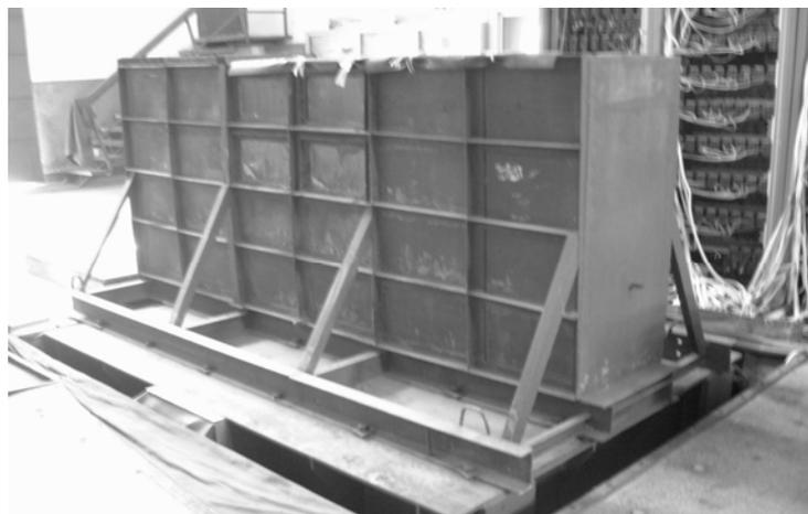
Fig 1 Model box on shaking table
