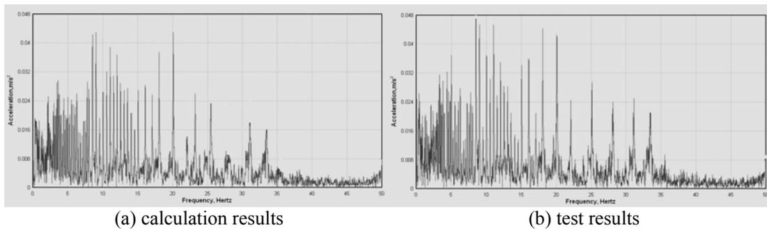
Fig.6 maximum z-acceleration FFT in loading mode 2
