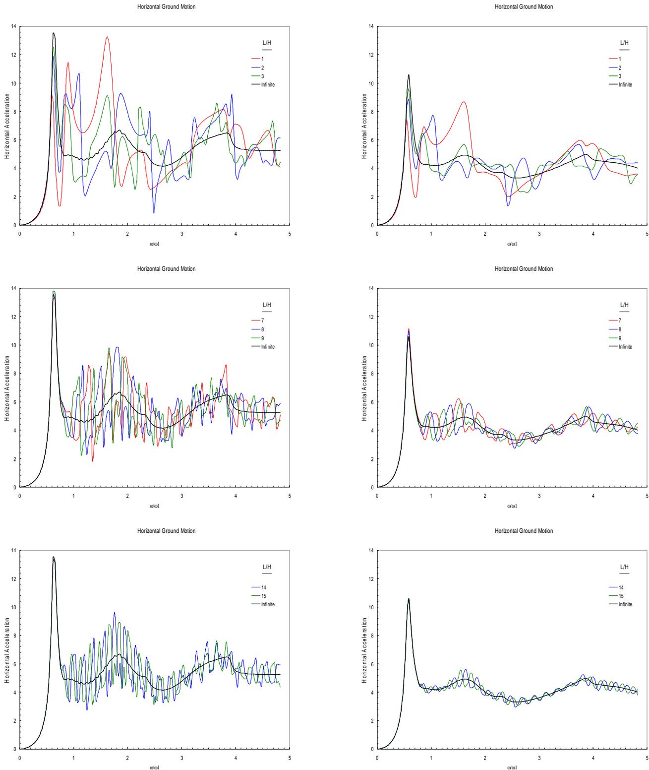
Figure 4 Horizontal acceleration at dam crest due to horizontal ground motion for different values of L/H
