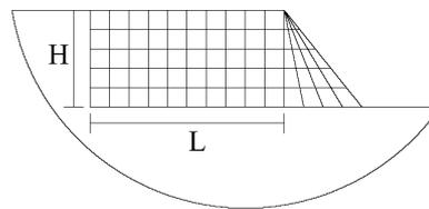
Figure 3 Discretization of dam-finite reservoir-foundation system for the case of  $L/H=2$
