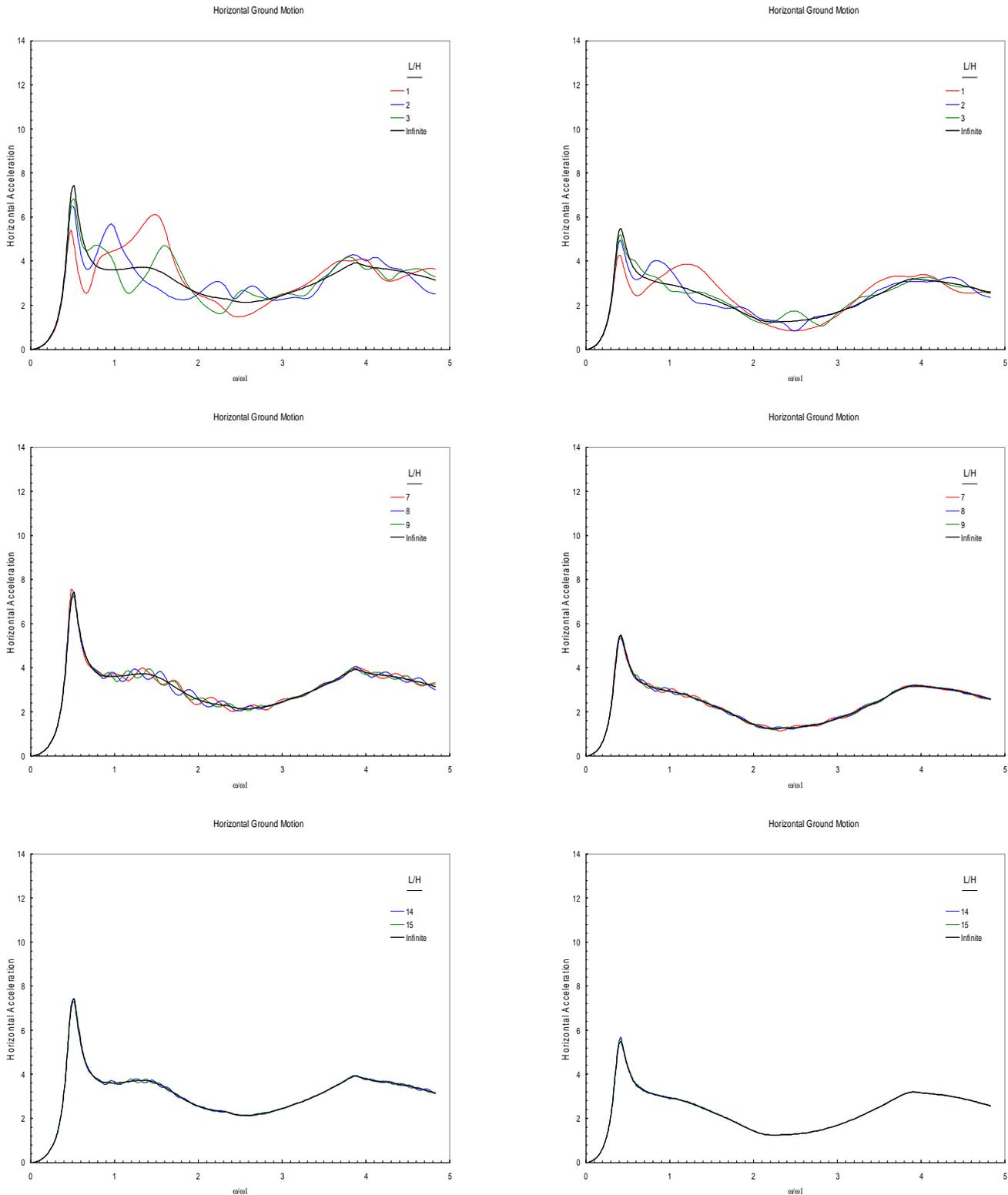
Figure 5 Horizontal acceleration at dam crest due to horizontal ground motion for different values of L/H
