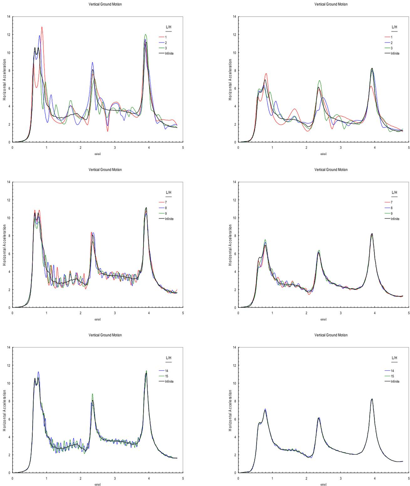
Figure 6 Horizontal acceleration at dam crest due to vertical ground motion for different values of  $L/H$
