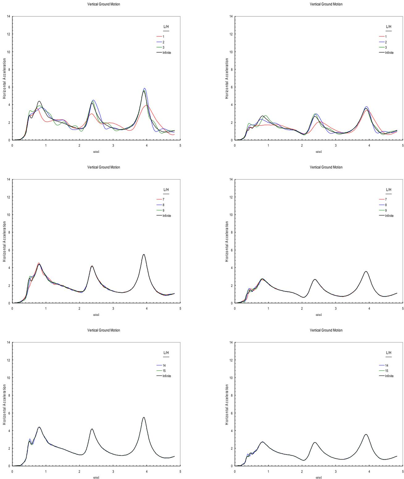
Figure 7 Horizontal acceleration at dam crest due to vertical ground motion for different values of L/H
