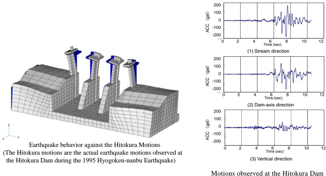
Figure 9 Earthquake behavior against the Hitokura motions
