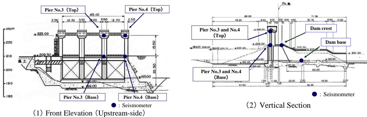
Figure 1 Shape of the spillway analyzed and location of seismometers
