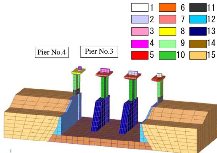
Figure 3 3-D dynamic analysis model (from down-stream side)
