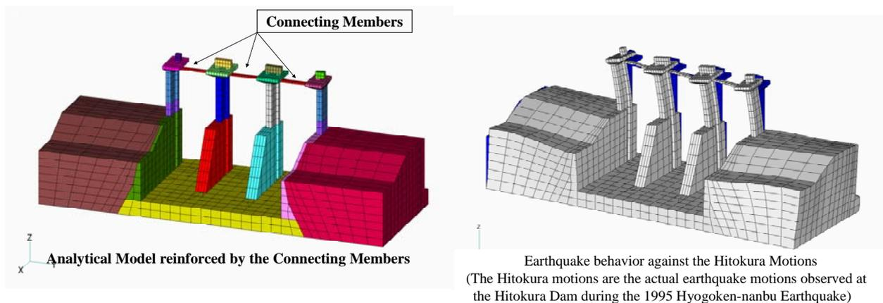
Figure 10 Countermeasures to reduce earthquake relative displacement
