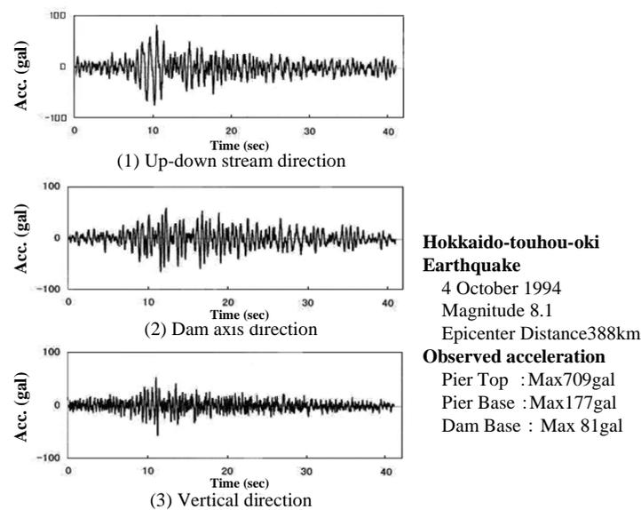
Figure 2 Acceleration time histories recorded at the bottom of dam in the 1994 Hokkaido-touhou-oki Earthquake, which are used as input motions for the 3-D reproduction analysis
