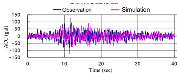
(1) Acceleration at the bottom of the No.4 Pier (Dam Axis)
