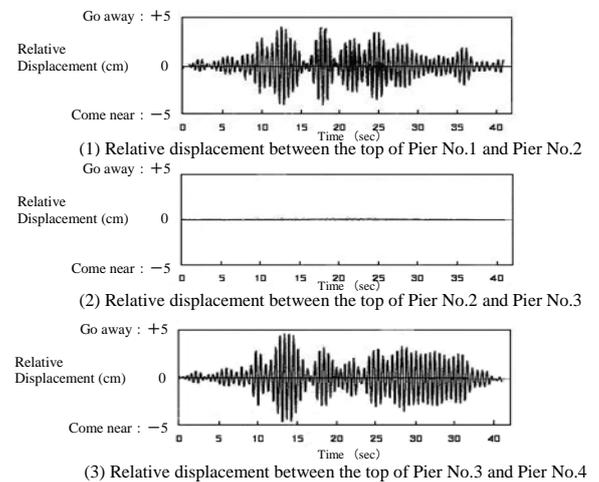
Figure 8 Relative displacement between the top of piers
