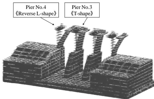
The Pier No.4 is the reverse L-shape and thin, and the Pier No.3 is the T-shape and thick. Therefore, the earthquake behaviors of these piers will become different from each other, and the relative displacement will appear by the earthquake motions. Maximum relative displacement between the top of Pier No.3 and Pier No.4 during the 1994 Hokkaido-touhou-oki Earthquake was estimated to be 4.9cm.
