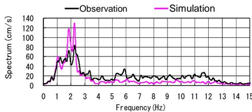
(2) Spectra at the bottom of the No.4 Pier (Dam Axis)
