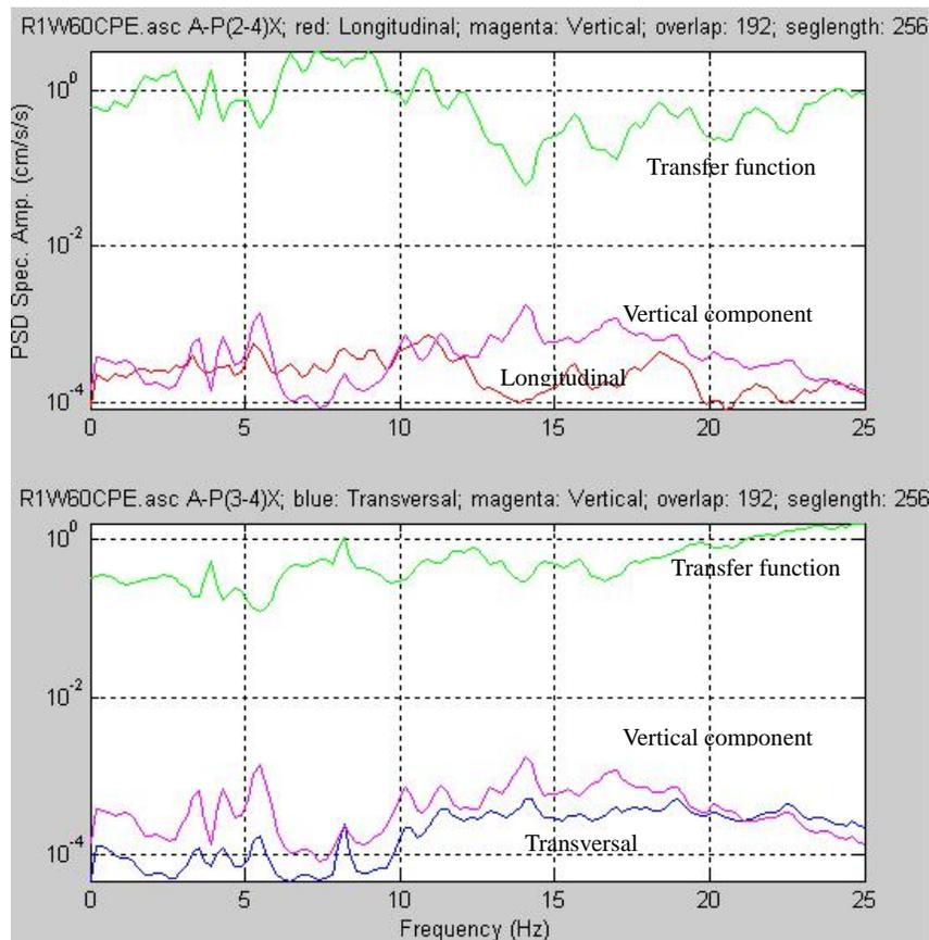
Figure 7 Fourier transform of signals at dam center. In both graphs, the upper line represents the Transfer Function obtained dividing the horizontal component by the vertical one.
