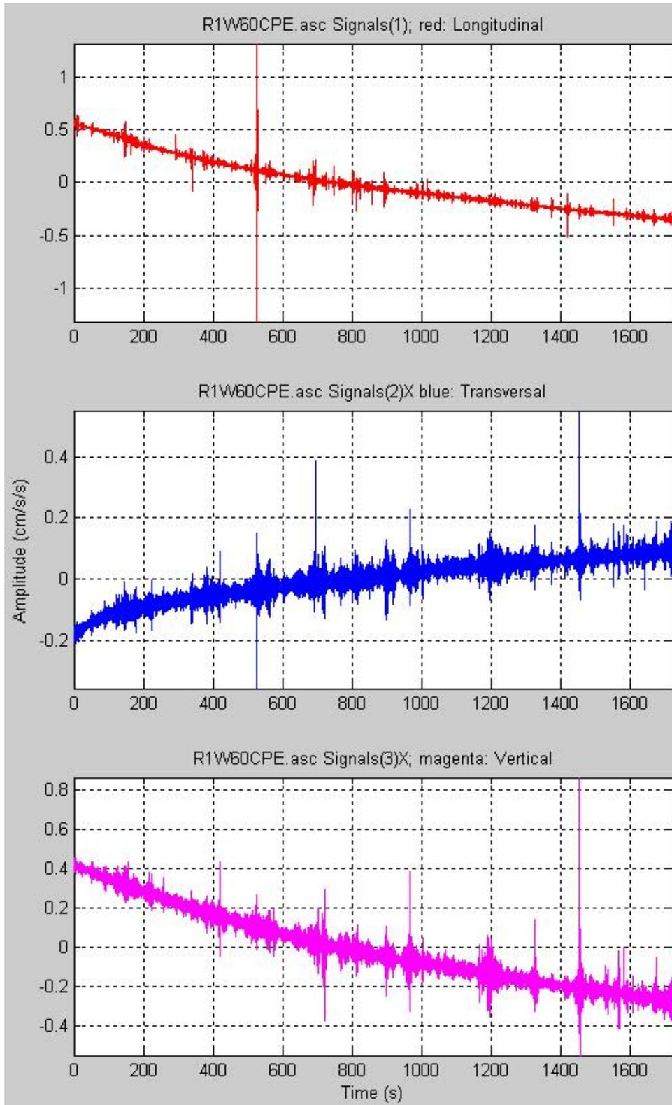
Figure 6 Graphs of time signals registered at dam center showing the three components.
