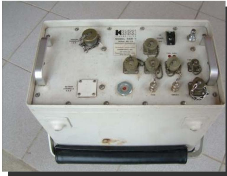
Figure 4 Kinometrics SSR-1 six channel recorder
