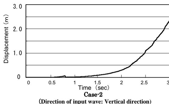
Figure 12 Time history of relative displacement of joint at the center of dam base when the acceleration wave is input in the vertical direction
