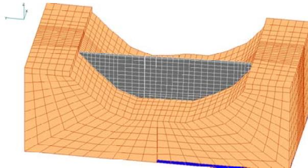
Figure 9 Displacement behavior of dam and fault when the acceleration wave is input in the horizontal stream direction
