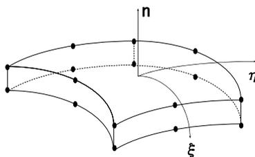
Figure 5 Structure of 3-D joint element
