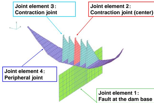
Figure 4 Distribution of the fault, the contraction joints, and the peripheral joint
