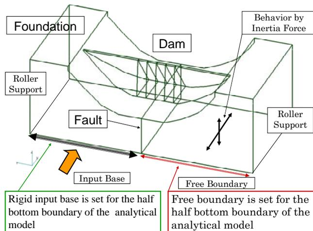
Figure 7 Boundary condition of 3-D analysis model
