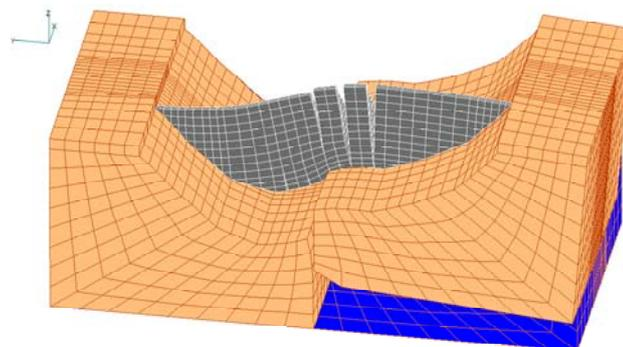
Figure 11 Displacement behavior of dam and fault when the acceleration wave is input in the vertical direction
