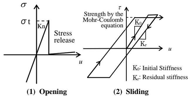
Figure 6 Mechanical characteristics of 3-D joint element
