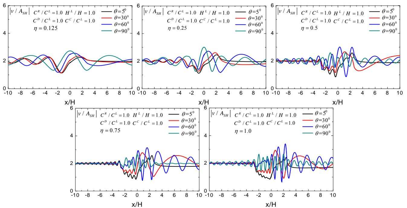
Figure 3 Surface displacement amplitudes of dam on homogeneous half-space
