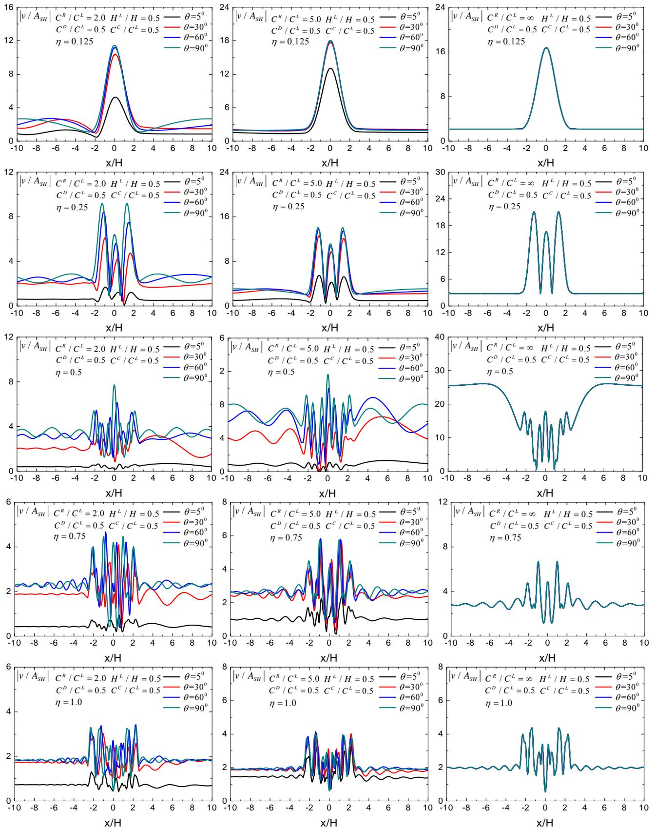
Figure 4 Surface displacement amplitudes of dam on layered half-space
