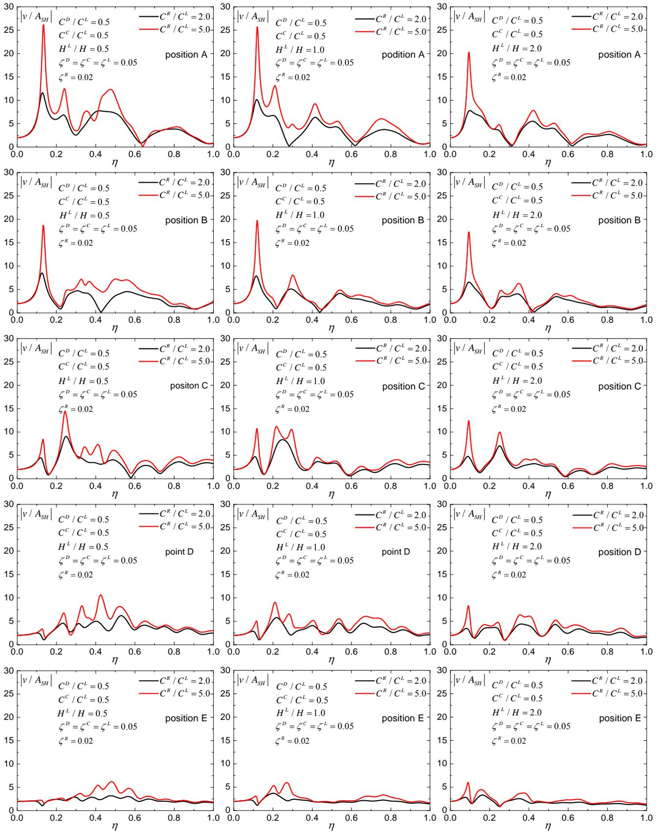
Figure 5 Spectral Amplification of dam on layered half-space
