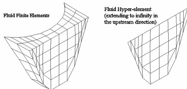
Figure (2) – Discretization of the reservoir domain by fluid finite elements and the fluid hyper-element (only coarse mesh)
