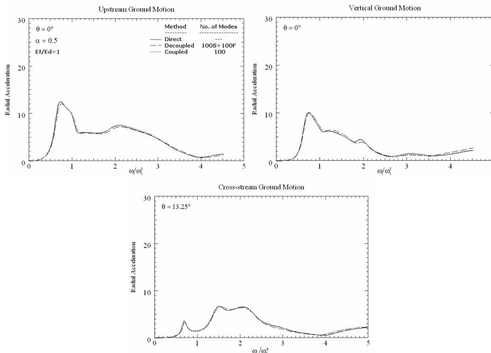
Figure (4) - Frequency-response functions by applying the coupled and the decoupled modal approach.
