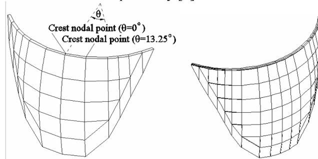
Figure (1) – Discretization of the dam body (coarse mesh and fine mesh)
