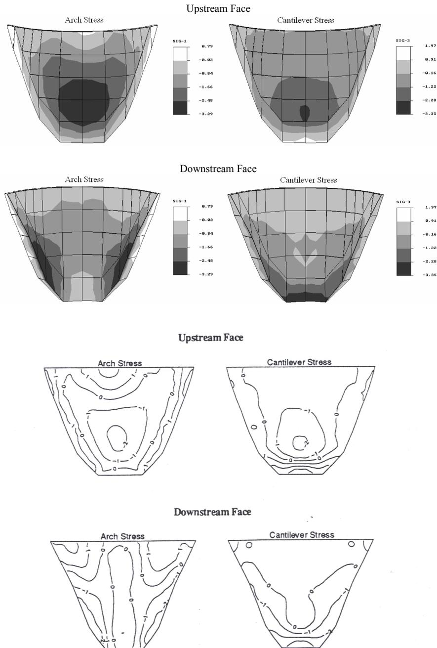
Figure (7) - Envelope values of the maximum arch and cantilever stresses (in MPa) due to upstream, vertical and cross-stream components, simultaneously, of Taft ground motion (above: present study; below: the work of Tan and Chopra [1])
