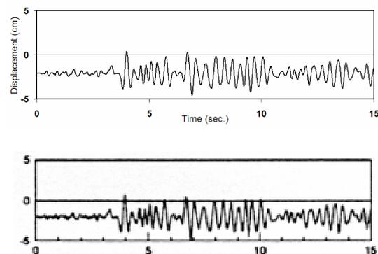
Figure (6) - Displacement response of mid-crest point of Morrow Point Dam (above: present study; below: the work of Tan and Chopra [1])
