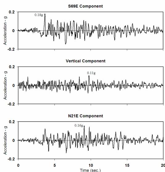
Figure (5) – Ground motion at Taft Lincoln School Tunnel, Kern County, California, earthquake 21 July 1952
