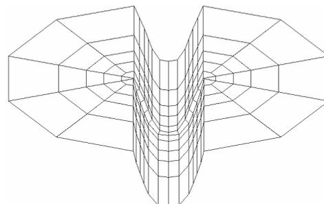
Figure (3) – Boundary element discretization of foundation rock (only coarse mesh)
