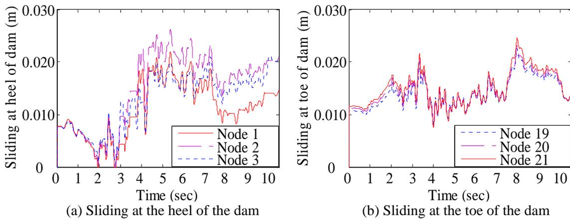
Figure 10 Sliding at the base of the dam for Scenario C
