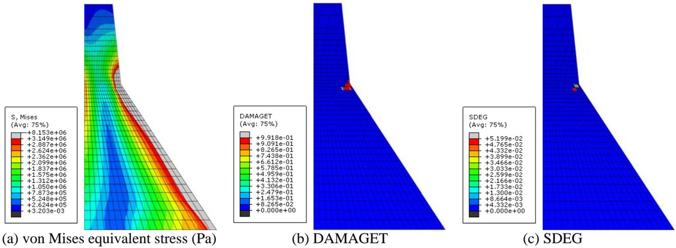
Figure 6 Contours of peak stress distribution and damage of the Koyna dam for Scenario B at 4.208 sec
