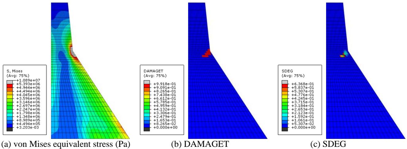
Figure 7 Contours of peak stress distribution and damage of the Koyna dam for Scenario C at 4.427 sec
