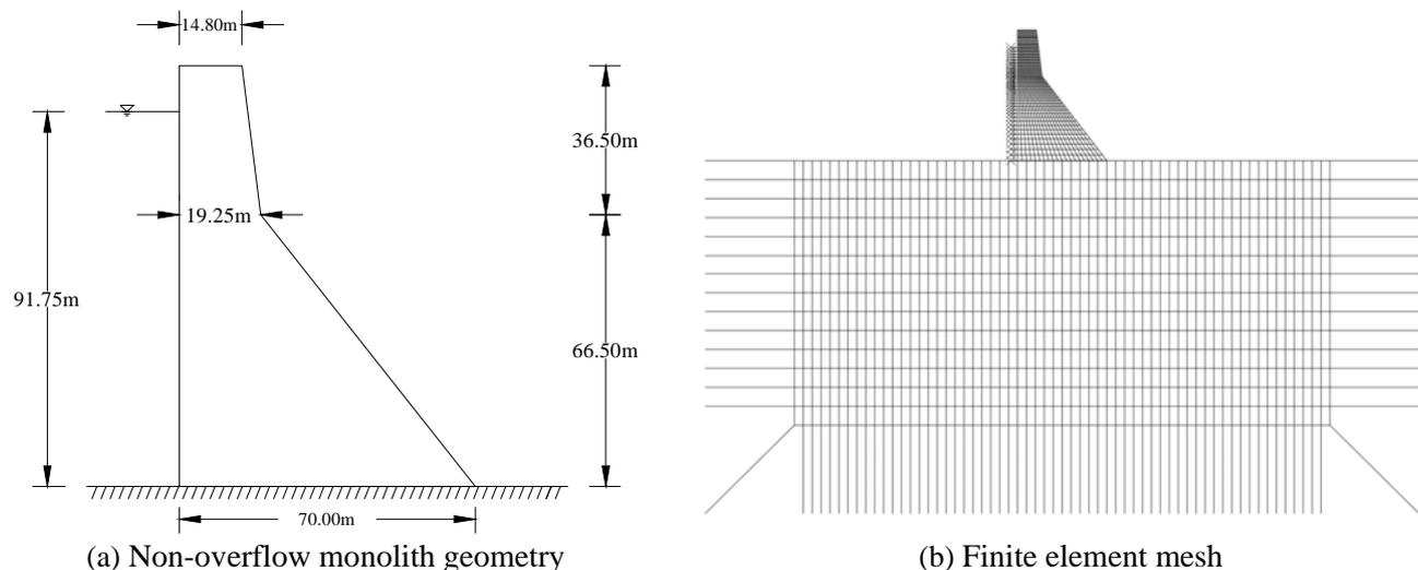
Figure 2 The numerical model of the Koyna dam
