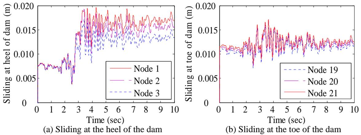
Figure 9 Sliding at the base of the dam for Scenario B
