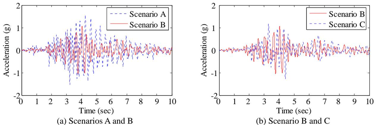
Figure 4 Comparison of horizontal crest acceleration responses
