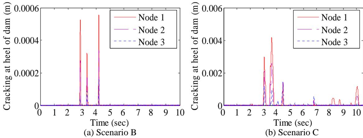
Figure 8 Cracking at the heel of the dam
