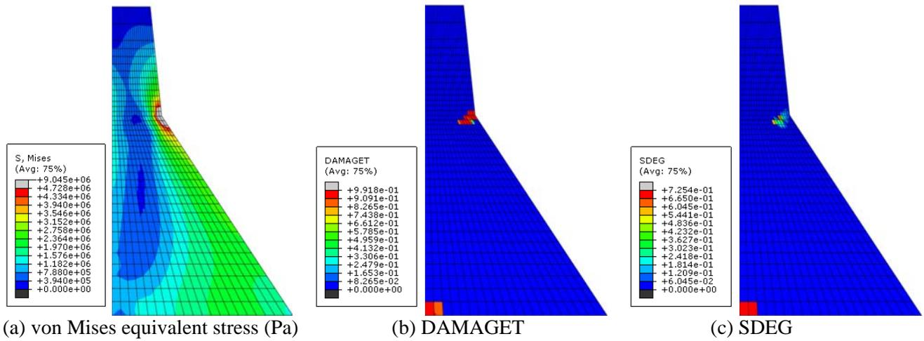
Figure 5 Contours of peak stress distribution and damage of the Koyna dam for Scenario A at 4.790 sec
