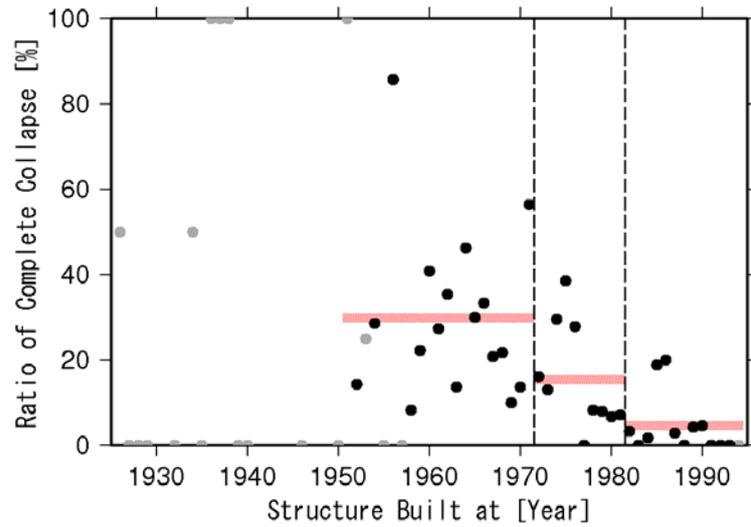
Figure 1 Damage ratio of RC structure buildings in 1995 Hyogo-ken Nanbu Earthquake.
