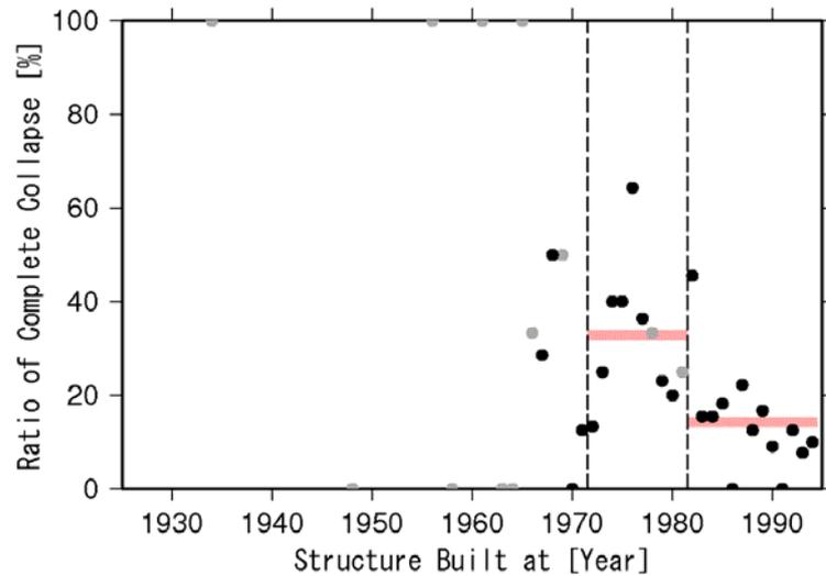
Figure 2 Damage ratio of steel structure buildings in 1995 Hyogo-ken Nanbu Earthquake.
