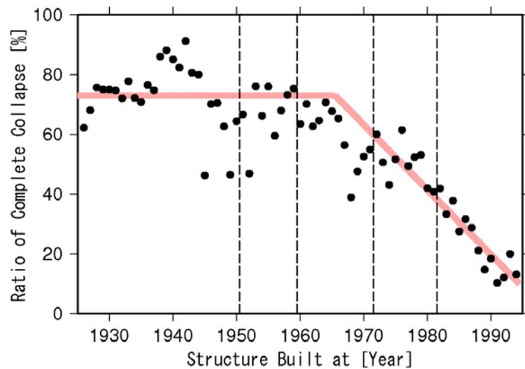
Figure 3 Damage ratio of wooden houses in 1995 Hyogo-ken Nanbu Earthquake.
