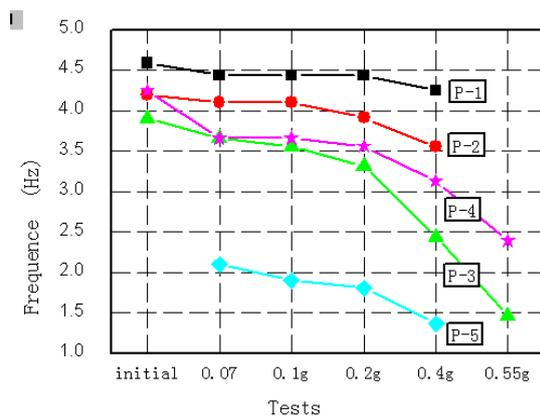
Figure 3 Natural frequency on Y direction
