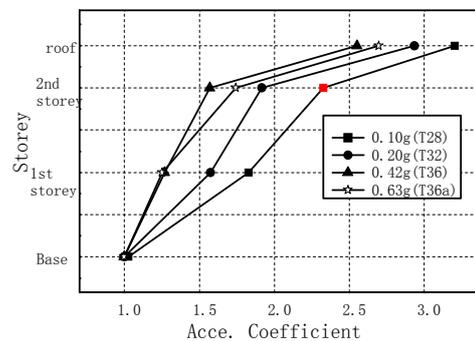
Figure 6 Acceleration coefficient of Pasadena record tests in Phase 3
