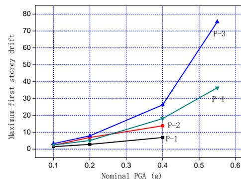
Figure 8 Maximum first storey drift in Phase 1~4
