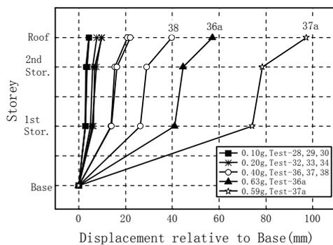
Figure 7 Max. Disp. relative to base in Phase 3
