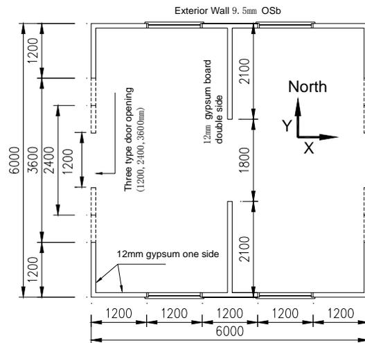
Figure 2 Main floor plan
