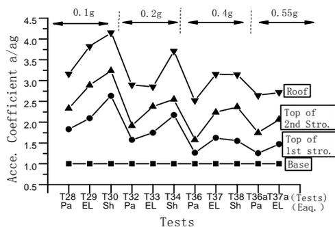
Figure 5 Acceleration coefficient in Phase 3
