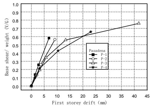
Figure 10 Capacity spectra of Pasadena earthquake tests in Phases 1~4
