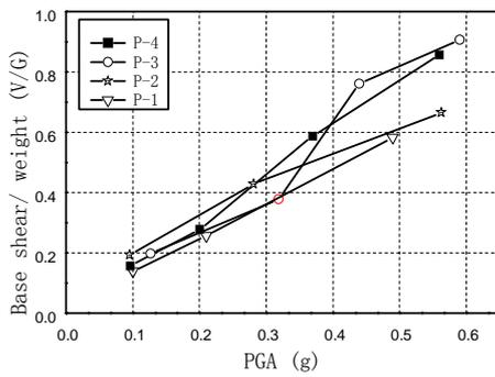
Figure 9 Max. base shear / total weight in Phase 1~4
