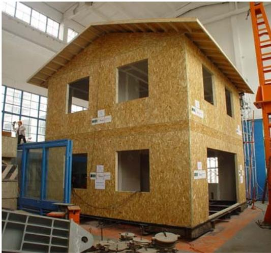
Figure 1 Specimen of Shake table test
