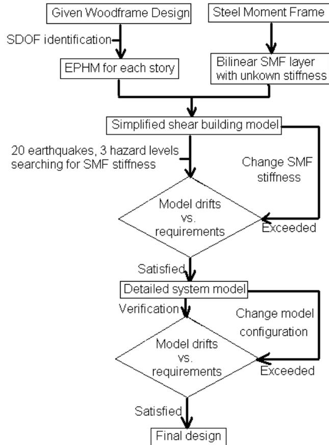
Figure 1 PBSD procedure used in this study
