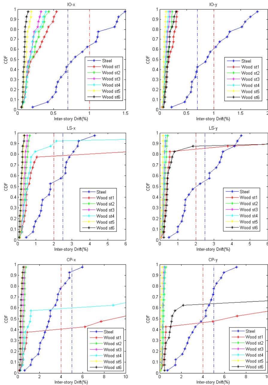
Figure 5 Maximum inter-story drift distributions in both directions
