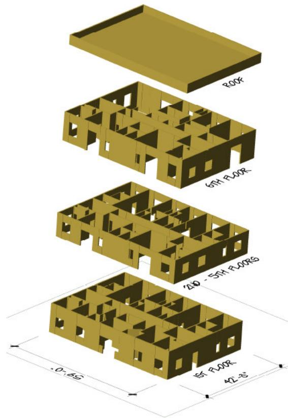
Figure 2 3-D of Capstone building (upper six stories of wood)
