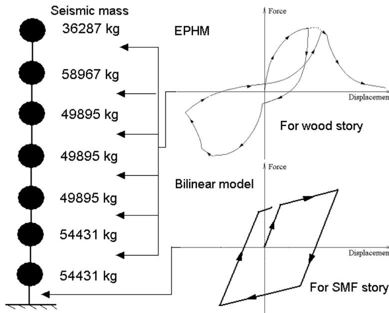
Figure 3 Shear building model simplification
