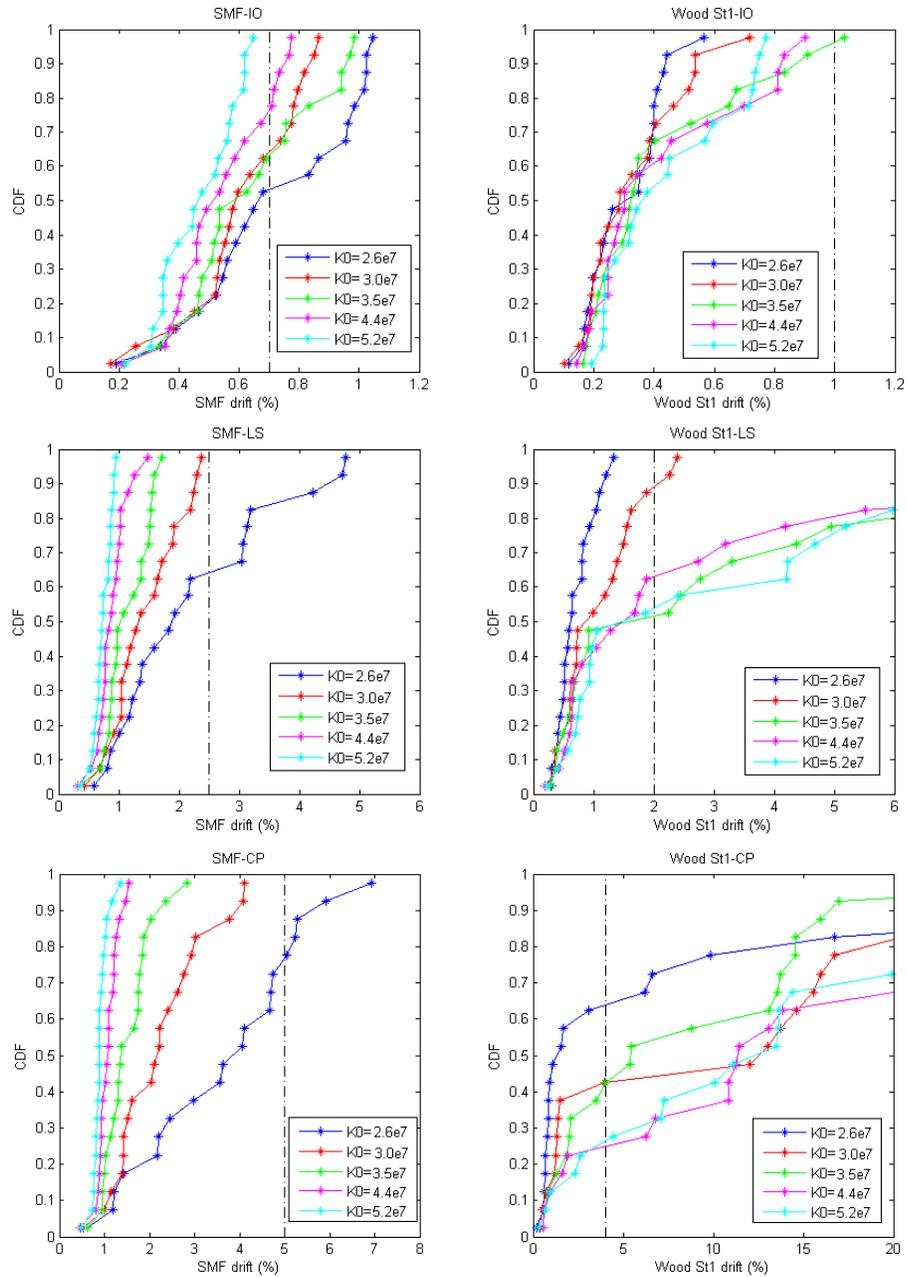
Figure 4 Maximum inter-story drift distribution for steel and wood (x-direction)
