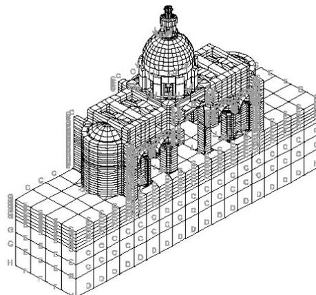
Figure 2 F.E.M. of the substructure and of its foundation soil
