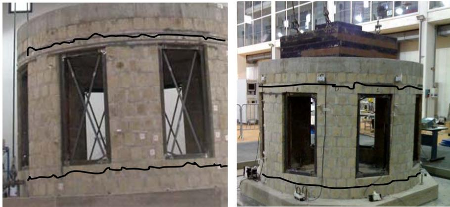
Figure 7 Location of the cracks for the model reinforced with frames and braced frames
