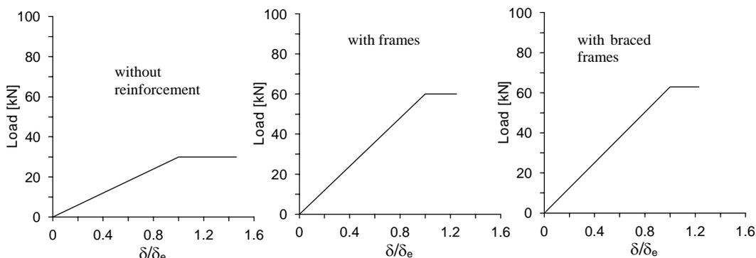
Figure 13 Horizontal load versus horizontal normalized displacement
