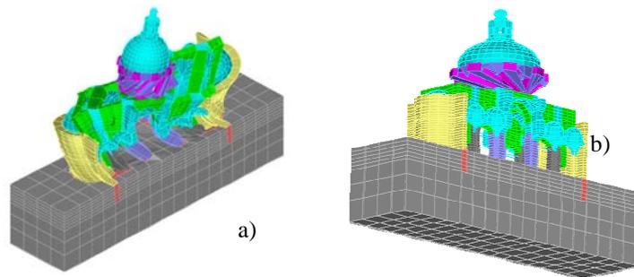
Figure 5 Two vibration mode obtained by the identified model
