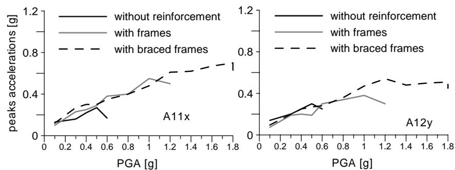
Figure 8 Peaks of response in terms of acceleration in two measure points on the top of the models
