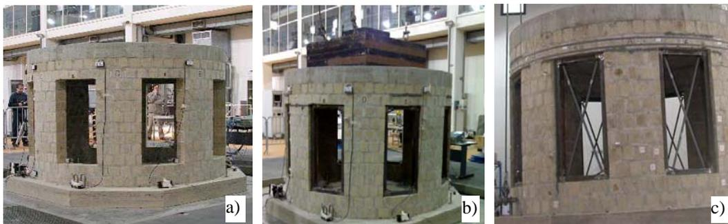
Figure 6 Model in the absence of reinforcement (a), model strengthened with frames (b) and with braced frames (c).
