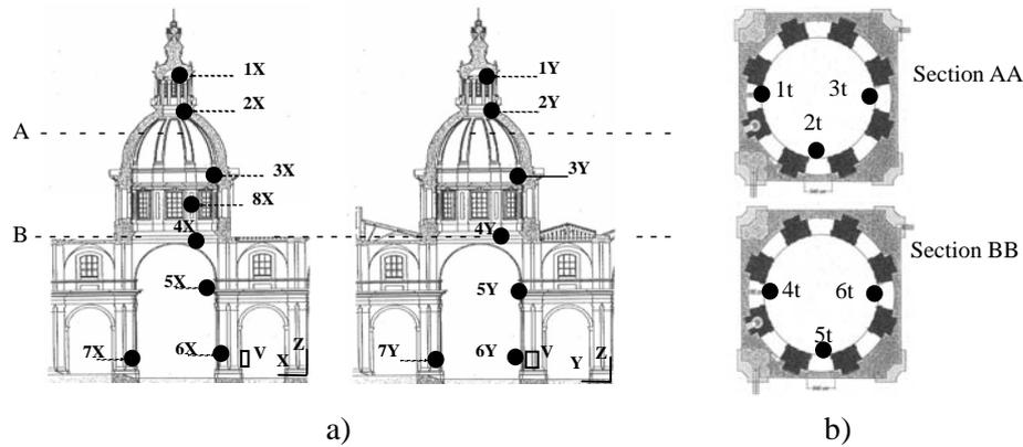
Figure 3 Measurement network for detecting lateral (a) and torsional (b) response
