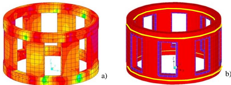
Figure 11 Stress state (a); model of the system in the damaged state (b)
