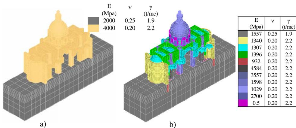
Figure 4 Model before (a) and after (b) the calibration
