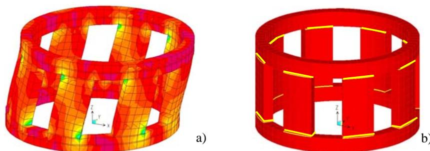
Figure 10 Stress/ strain state (a); model of the system in the damaged state (b).
