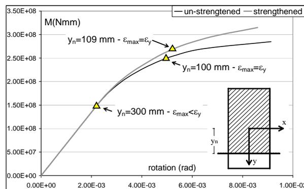
Figure 3 Test beam: moment-rotation curve
