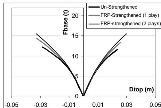
Figure 9 Pushover curves: effect of the FRP-strengthening
