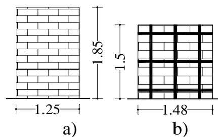
Figure 4 Geometry of the examined masonry panels: a) un-strengthened panel, Fantoni, 1981; b) FRP-strengthened panel, Marcari, 2005
