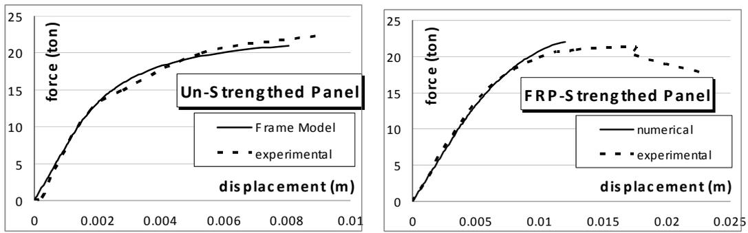
Figure 5 Horizontal load vs. top displacement curves
