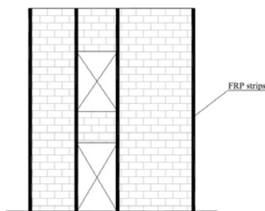
Figure 8 Configuration of the FRP-strengthening system
