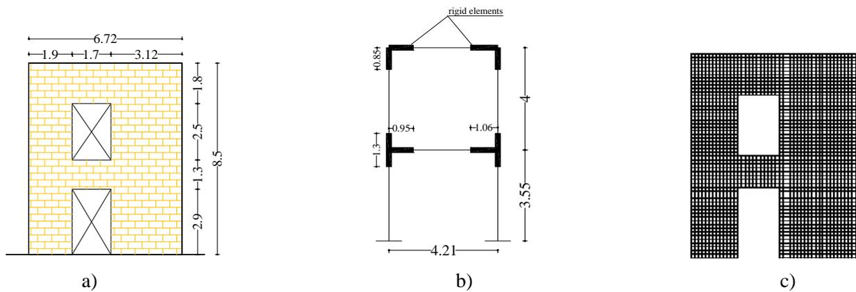
Figure 6 Masonry façade: a) geometry; b) equivalent frame; c) FE model A
