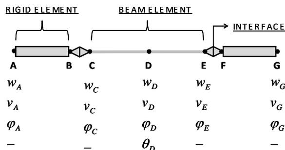
Figure 1 Proposed finite element
