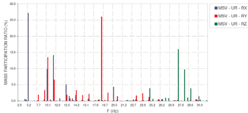
Figure 7 Mass participation ratios for each of the vibration modes and the main directions (XX, YY and ZZ).
