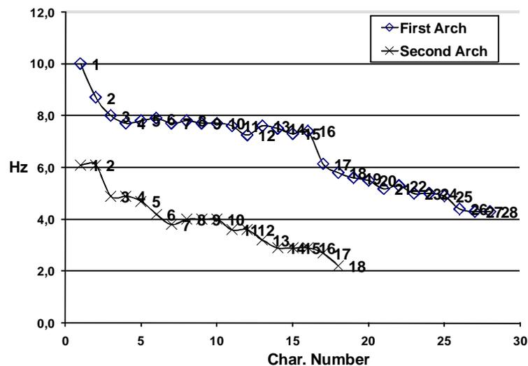
Figure 3 Variation of the first resonance frequency.
