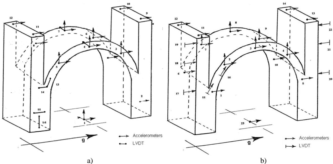
Figure 1 Sensors layout in masonry barrel vault specimens 1 (a) and 2 (b).
