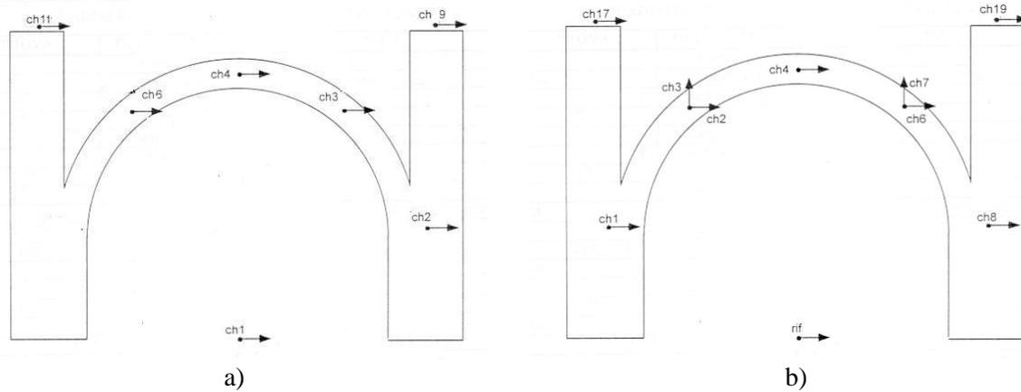
Figure 2 Sensors layout on the arch surface for specimen 1 (a) and specimen 2 (b).
