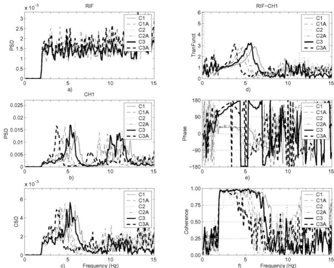
Figure 4 Comparison between characterization obtained during the preliminary phases (light load and pink noise) of specimen 2 test
