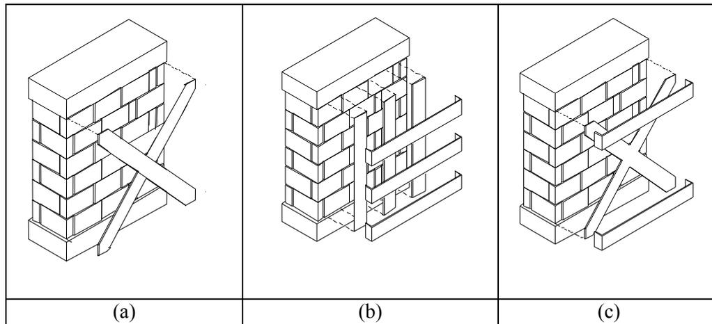
Figure 2 (a) Clay brick walls strengthened with cross layout (Zhao et al. 2003; Santa Maria et al. 2006), Tuff masonry walls strengthened with grid (b) and cross (c) layout (Marcari et al. 2007)
