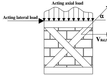
Figure 1 Mechanical model for FRP shear contribution in diagonal layout
