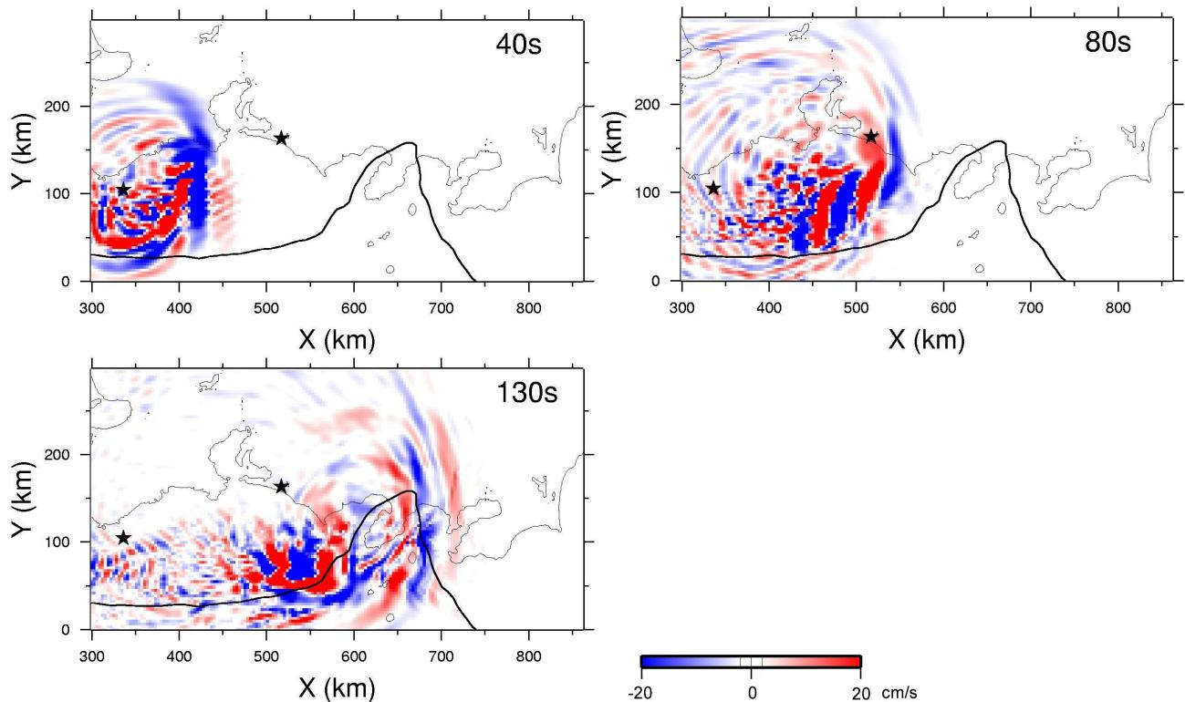
Fig.9 Snapshot of velocity Y (N29W) component of Tonankai-Tokai coupled earthquake
