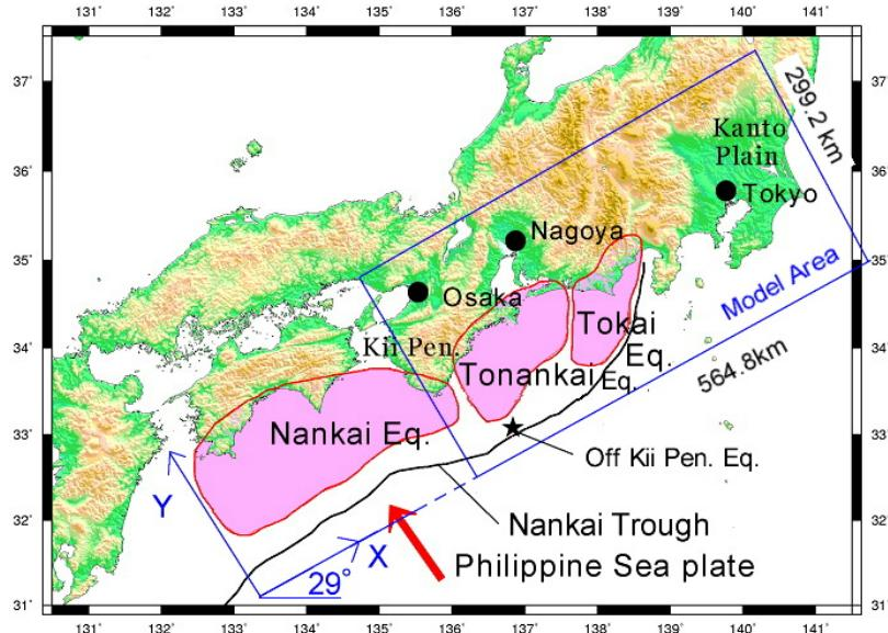
Fig.1 M8 earthquakes along Nanakai trough, the epicenter of the 2004 off the Kii peninsula earthquake and model area for FEM calculation
