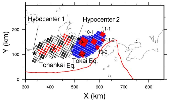
Fig.8 Source Model of Tonankai-Tokai coupled earthquake
