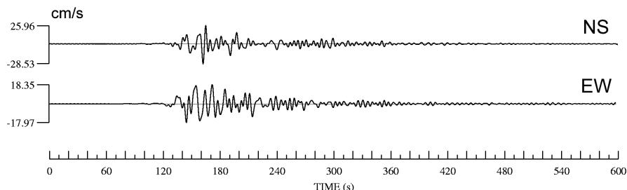
Fig.10 Calculated velocity of Tokai-Tonankai coupled earthquake at SJK
