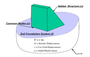
Figure 1 Soil Structure interaction model
