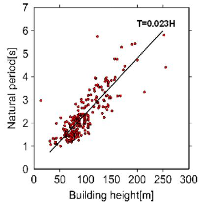
Figure 9 Relationship between the natural period of high-rise building (T) and building height (H) in the Osaka plain. Linear relationship with proportionality coefficient of 0.023 fit the data well.
