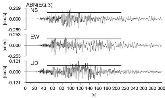
Figure 3 Example of the velocity seismogram recorded at site ABN for EQ.3. The records are band-pass filtered from 0.1 to 3Hz. Solid lines indicate the segment of the record (163.64 s) used for the spectral analysis.
