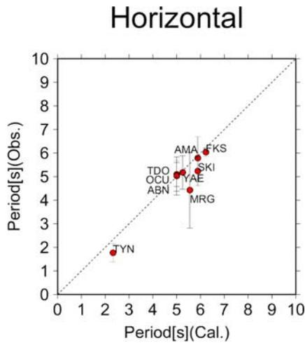
Figure 6 Comparison of the predominant periods of Love waves calculated for the 1-D velocity model at CEORKA sites (Cal.), with the observed ones (Obs.) for the horizontal component of the seismograms. Vertical bars denote the range of the standard deviation.
