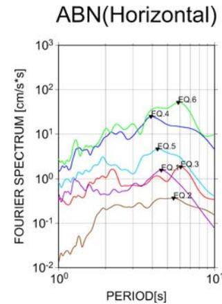
Figure 4 Fourier spectra of horizontal component for earthquakes observed at site ABN. Reverse-triangles indicate the predominant period for each earthquake.
