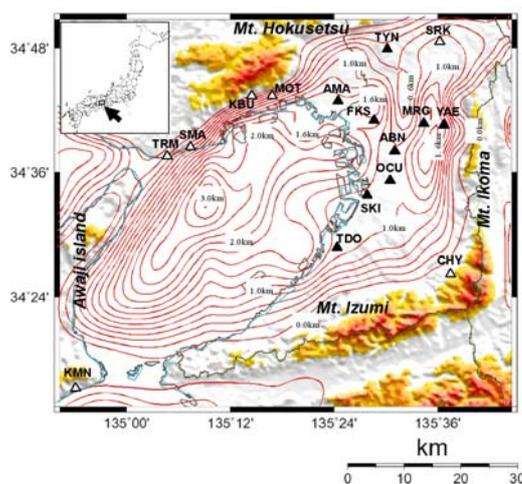
Figure 1 The Osaka basin, western Japan, model (Miyakoshi et al., 1999). Triangles showing locations of the strong ground motion observation stations maintained by CEORKA. Filled triangles denote CEORKA sites used in this study.
