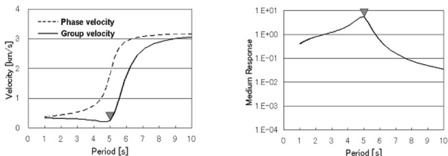
Figure 5 Examples of the theoretical dispersion curves (left) and the medium response (right) of the fundamental mode of Love wave, calculated for 1-D velocity model at site ABN extracted from the Osaka basin model (Miyakoshi et al., 1999). The theoretical dispersion curves are shown for the phase velocity (broken line) and the group velocity (solid line). Reverse-triangle denotes the period of the Airy phase (the minimum group velocity).
