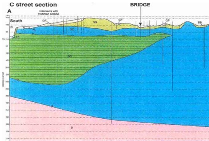
Figure 1: The geological cross-section along North-South direction at C-OM site. The vertical lines represent the shallow borehole locations around the bridge site. The bridge location is marked with an arrow (Adopted from Combellick, 1999).
