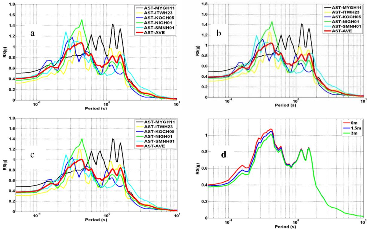
Figure 6: The plot of 5 % damped response spectra at the surface motions for five selected input motions for three soil conditions: (a) unfrozen soil and seasonally frozen soil of thickness (b) 1.5 m and (c) 3.0 m. Figure (d) compares the average value of response spectra for above three soil conditions.
