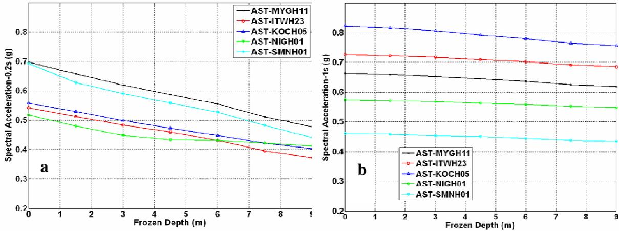
Figure 5: Effect of frozen depth on SA at (a) 0.2 sec and (b) at 1 sec for selected earthquakes scaled according to the AST –level hazard (7% probability in 75 years) at C-OM site.
