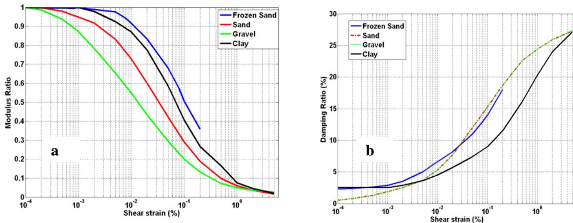
Figure 3: (a) The modulus reduction curves and (b) the damping ratio for three soil units (sand, gravel, clay) and frozen sand layer.
