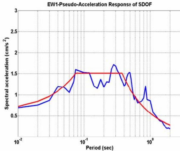
Figure 2: An example of scaling of horizontal motions of three recorded events from Kik-Net data. The blue and red lines are response spectra of scaled acceleration THs and target response spectra corresponding respectively for the C-OM site.
