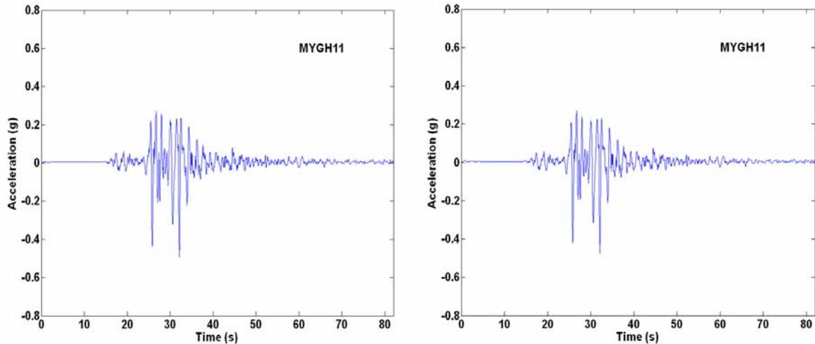
Figure 4. Computed time histories at the surface of C-OM site due to (left) unfrozen soil and (right) frozen soil of 3 m thick for MYGH11 event referred in Table 2.
