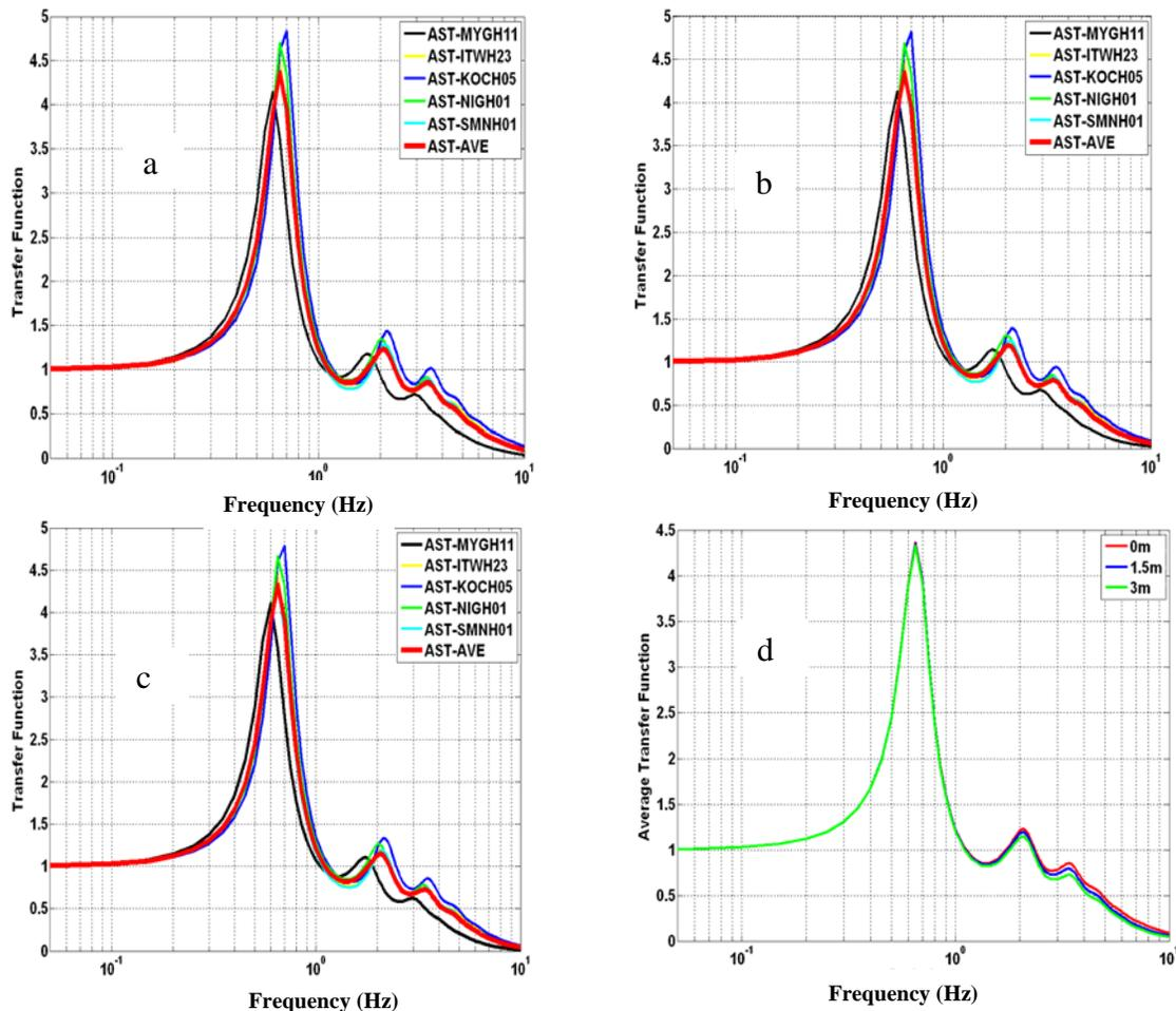
Figure 7: The plot of transfer function between the surface and bed rock motion for selected events as labeled in individual plots for three types of soil conditions: (a) unfrozen soil and seasonally frozen soil of thickness (b) 1.5 m and (c) 3.0 m. The solid red line in each plot indicates the average value of the transfer function. (d) Comparison between the average value of transfer functions for above three soil conditions.
